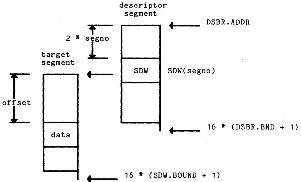
Figure 5-1. Main Memory Address Generation for Unpaged Segments
