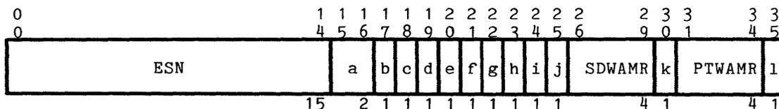
Odd word of Y-pair as stored by Store Central Processor Register (sopr),
