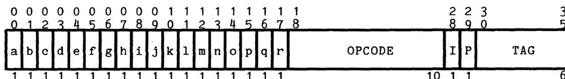
Odd word of Y-pair as stored by Store Central Processor Register (scpr), TAG = 20
