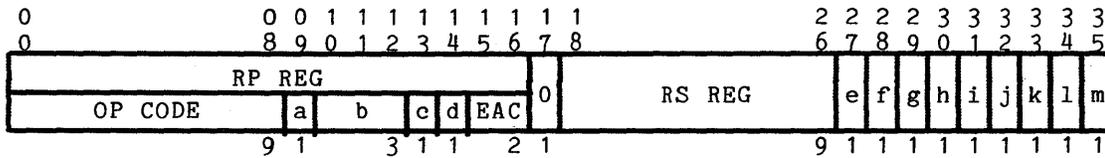
Odd word of Y-pair as stored by Store Central Processor Register (scpr), TAG = 40
