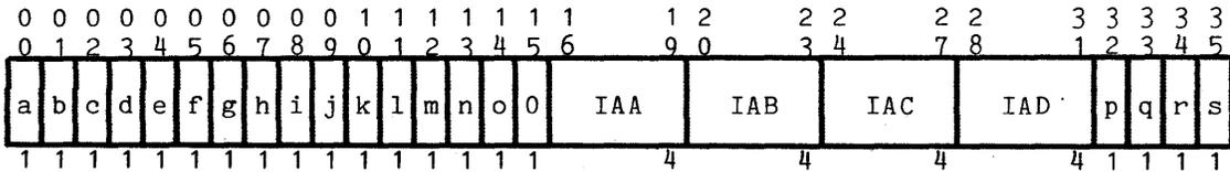
Odd word of Y-pair as stored by Store Central Processor Register (scpr), TAG = 01
