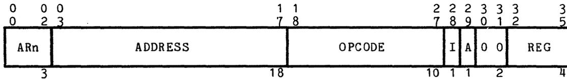
Figure 1. EIS Address Register Special Arithmetic Instruction Format
