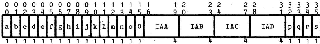
Odd word of Y-pair is stored by Store Control Processor Register (sopr), TAG = 01
