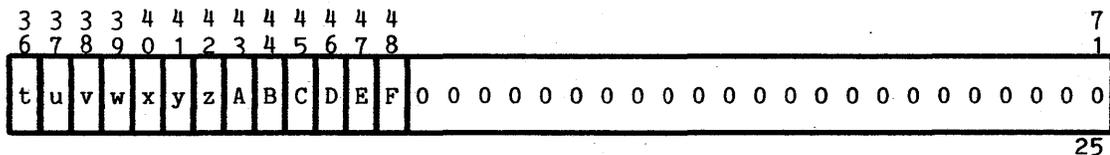
Figure 3-19. Fault Register (FR) Format - DPS 8M
