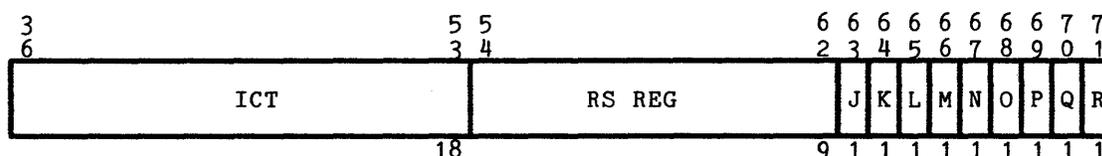
Figure 3-27. Decimal/Operations (DU/OU) History Register Format - DPS 8M
