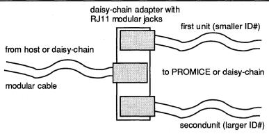
With the center jack's opening facing you, connect the master (unit 0 on a simplex or units 0 and 1 on duplex units) PromICE to the left connector and the slave (unit 1 on a simplex or units 2 and 3 for duplex units) PromICE to the right (the jacks that go to the PromICE will be facing away from you). Any number of PromICE units can be daisy chained in this way.
