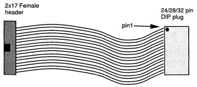
**WARNING:** CONNECTING THE CABLE INTO THE ROM SOCKET BACKWARDS WILL DAMAGE THE PromICE. Connect the other end of the cables to the PromICE. There is a 34 pin female IDC connector with a key. Insert it carefully on the back of the PromICE. If you are using a 16 bit or larger system, Make sure the byte order is set correctly.
