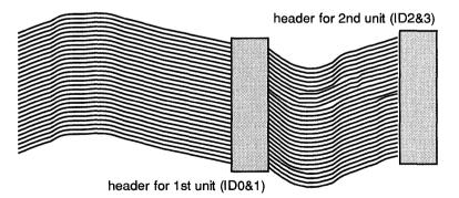
Two PromICE units can be daisy chained in this configuration. Connect the parallel adapter cable with the center header to the first PromICE (unit 0 on a simplex or 0 and 1 on duplex units). The header farthest away from the host connection should be connected to the second PromICE (unit 1 on a simplex or units 2 and 3 on duplex units).
