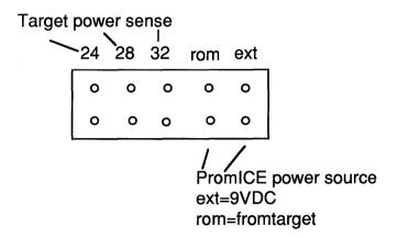
Set one jumper on either the "ext" pins for external power (preferred) or the "rom" pins for parasitic power (When using parasitic power, the PromICE takes its power directly from the target's ROM socket. No external power supply is connected to the PromICE).
