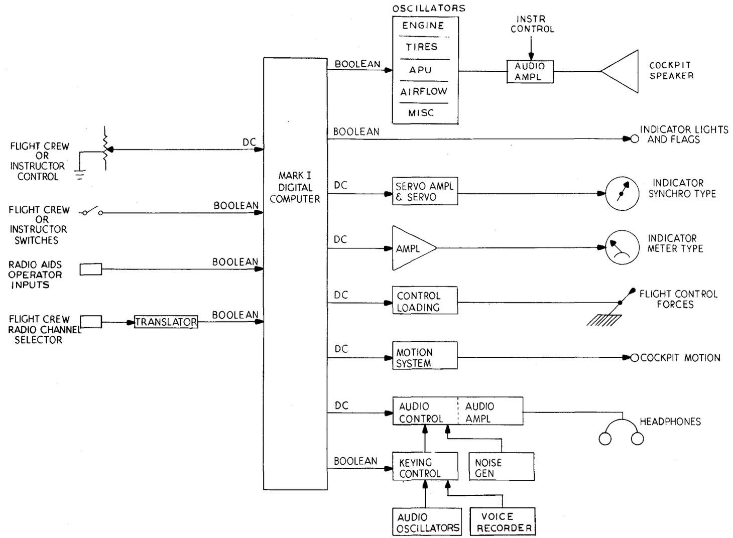
Figure 2 BLOCK DIAGRAM OF MARK I FLIGHT SIMULATOR
