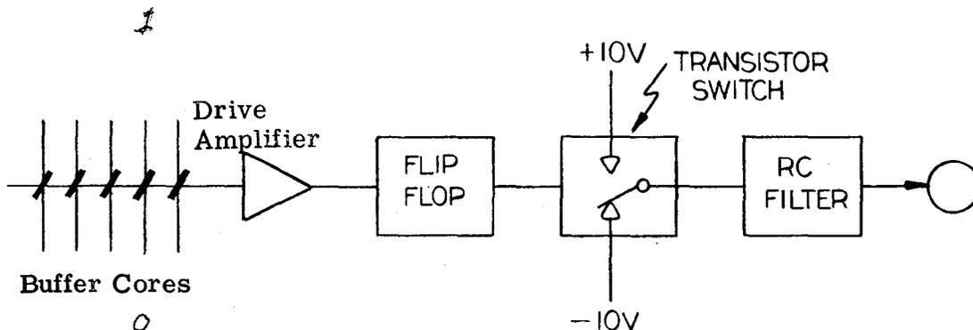
Figure 13 SIMPLIFIED DIAGRAM OF D-A CONVERTER
