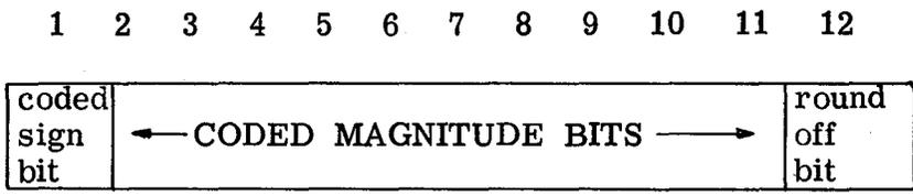
This 12th bit is generated by forming the one's complement of the 12th bit on the word in main core. That is, if the sign of the word in the main core is positive, the 12th bit transfers to the output register unchanged. If the sign of the word in the main core is negative, the complement of the 12th bit is transferred to the output register.
