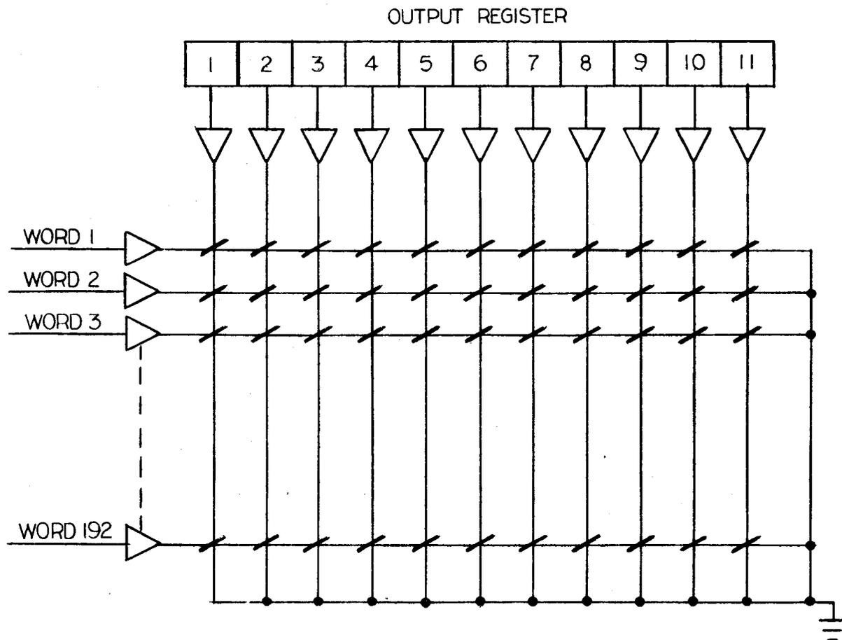
Figure 11 192-WORD BUFFER CORE AND OUTPUT REGISTER
