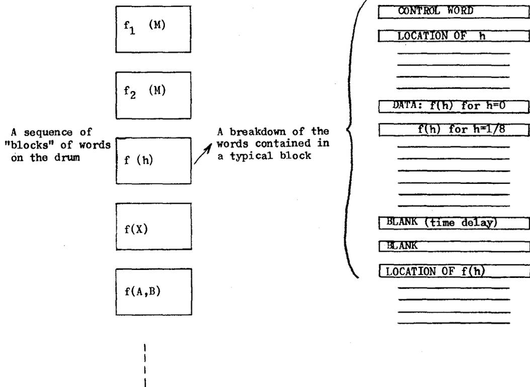
Figure 16 DRUM REPRESENTATION OF FUNCTION DATA
