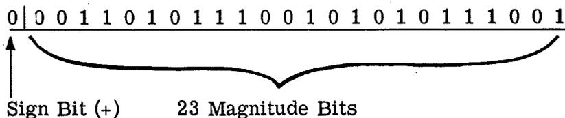
In the Mark I's fixed-point arithmetic, the decimal point is assumed to be to the left of the most significant bit; therefore, the magnitude of a number is always less than one. The largest magnitude that may be represented is .99999. . . . in decimal notation, or .111111 . . . . in binary notation. All numbers handled by the Mark I must be scaled with this fixed-point notation in mind.
