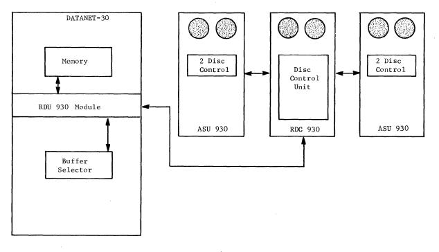
Figure 27. DATANET-30/RDC 930 Block Diagram
