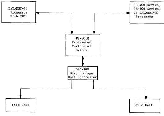
Figure 30. Typical PS-6010 Switch Application
