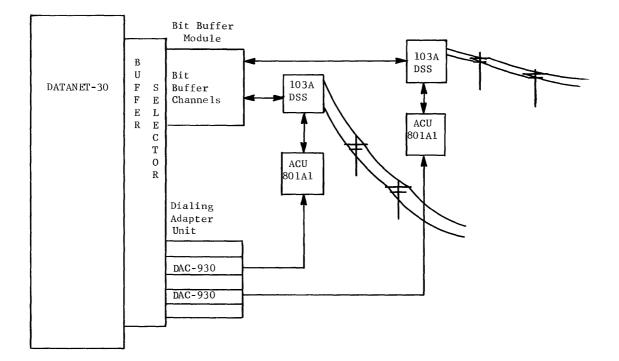
Figure 19. Dialing Adapter Units with Telephone Equipment and Bit Buffers
