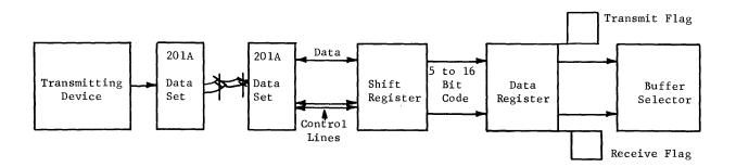
Figure 18. Character Buffer Channel Block Diagram
