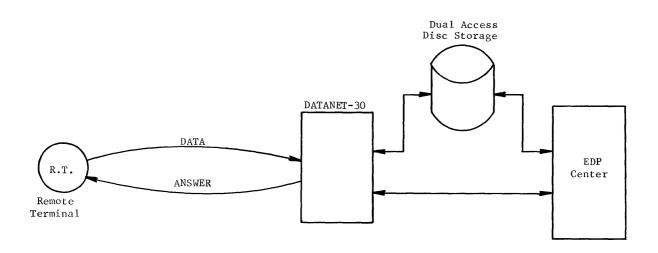
Figure 9. Remote Data Processing
