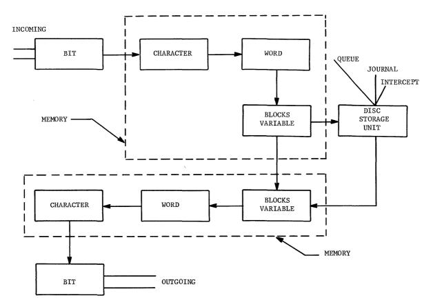
Figure 33. Data Flow Functional Block Diagram
