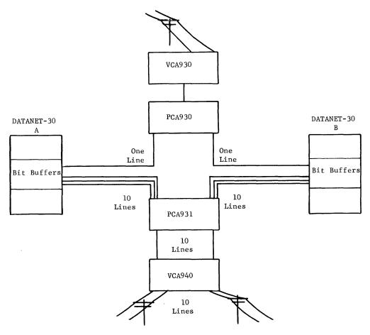
Figure 31. Parallel Channel Adapter Block Diagram
