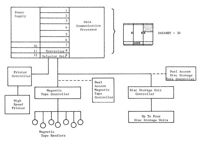
Figure 25. DATANET-30 with Controller Selector Unit and Peripheral Equipment
