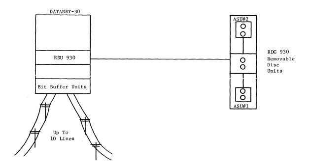
Figure 2. System with RDC 930 Units
