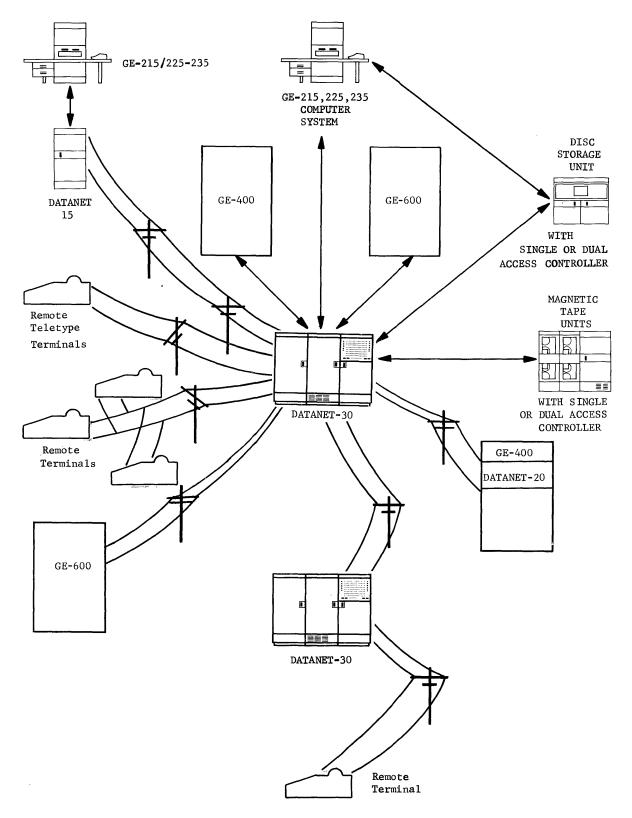
Figure 10. DATANET-30 System Components-Not a Typical System
