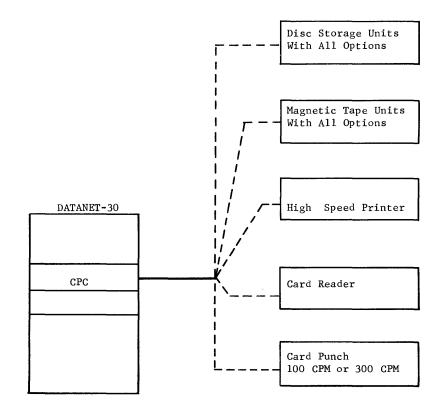
Figure 26. CPC Peripheral Equipment
