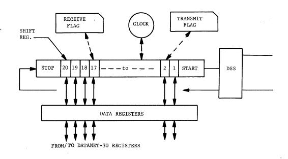
Figure 17. Word Buffer Channel Transmit and Receive
