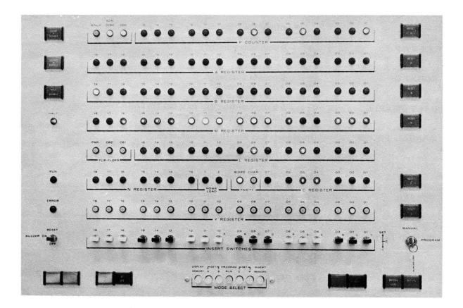
Figure 36. The Control Console
