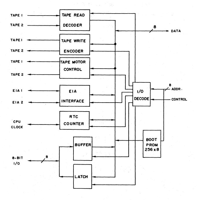
TAPE - EIA I/O MODULE SPECIFICATIONS
