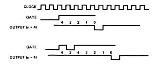
Figure 5. 8253 Timing Diagrams
