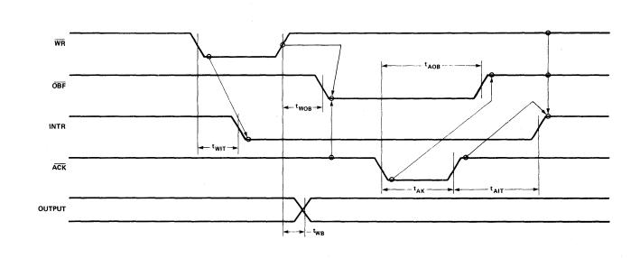
Figure 29. MODE 1 (Strobed Output)
