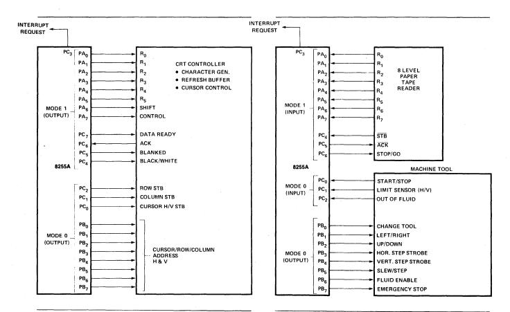
Figure 21. Basic CRT Controller Interface
