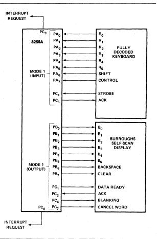
Figure 18. Keyboard and Display Interface
