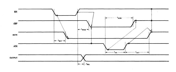
Figure 9. Mode 1 (Strobed Output)
