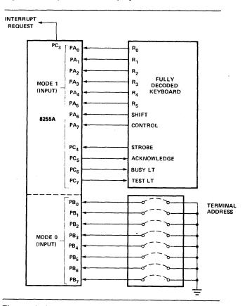
Figure 19. Keyboard and Terminal Address Interface
