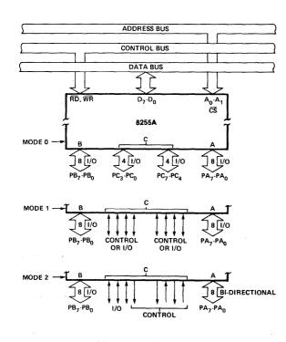
Figure 3. Basic Mode Definitions and Bus Interface
