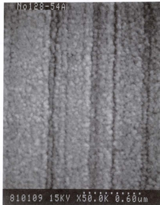
c) Ar at Cr sputtering: 0.4 Pa Ar at CoCrTa sputtering: 4.0 Pa
