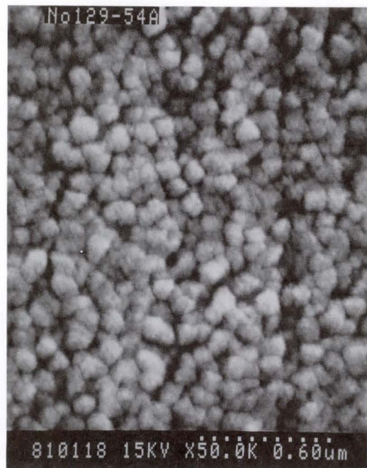
d) Ar at Cr sputtering: 4.0 Pa Ar at CoCrTa sputtering: 4.0 Pa
