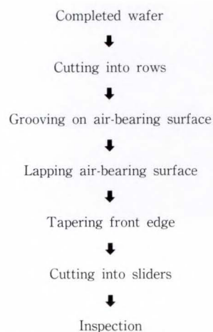
Fig. 23—Slider machining flow.
