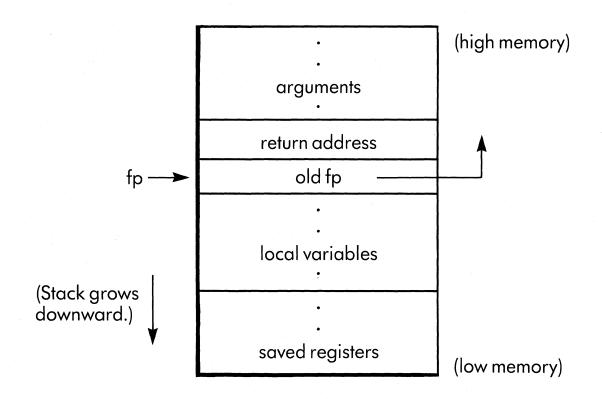
Figure 13-1. The Run-Time Stack (Stack Grows Down the Page, or From High Memory to Low Memory)
