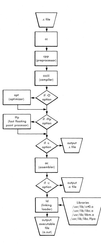
Figure 1-1. Path of a C Source File Through the Compiler
