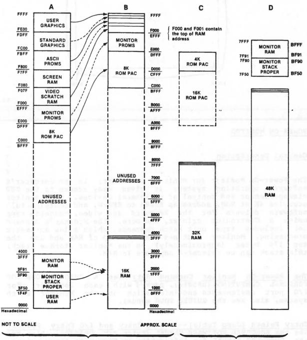
STANDARD CONFIGURATION (16K RAM + SK ROM PAC INSERTED) ALTERNATIVE CONFIGURATIONS (Drawn to Approximate Scale)
