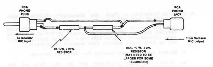
Figure 6 Attenuator Plug
