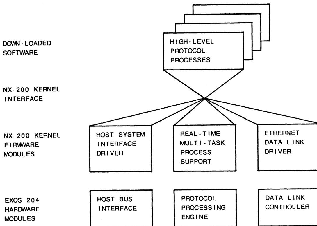
Figure 1-3: NX 200 Software Architecture
