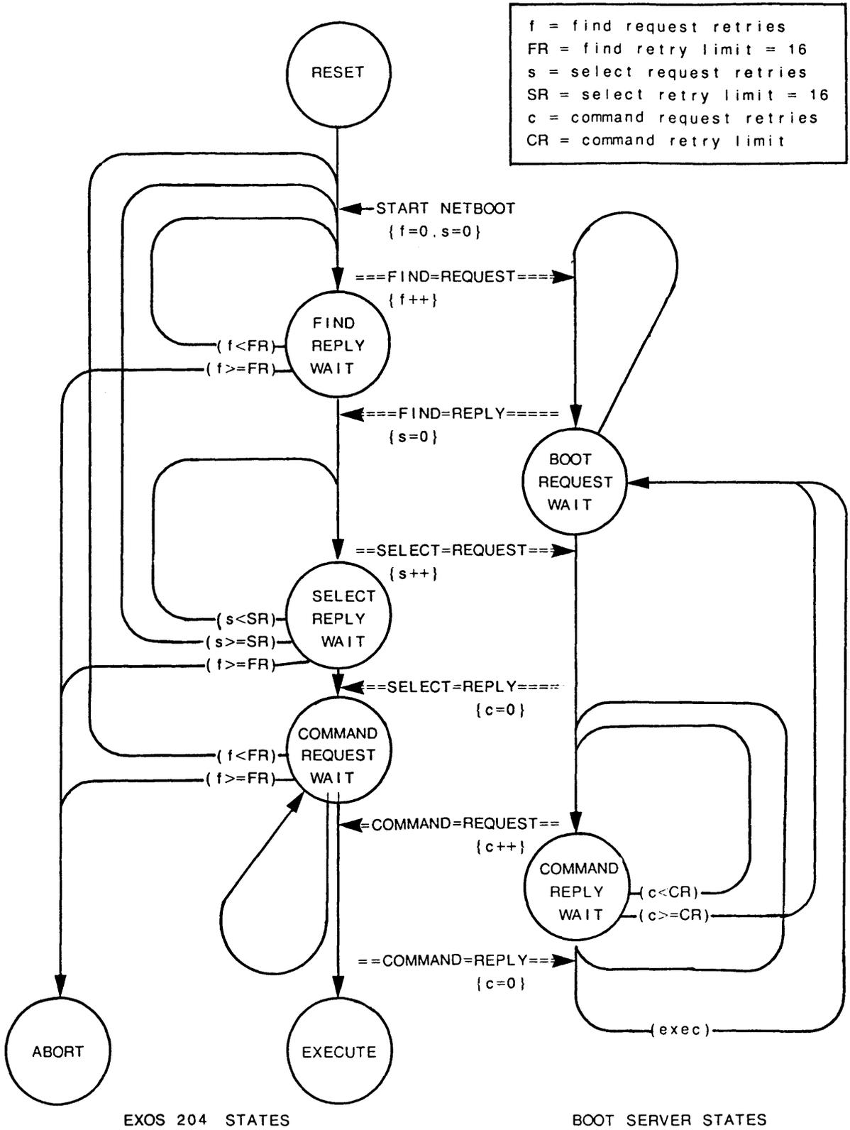
Figure 10-1: State Diagram of Network Bootstrap Protocol
