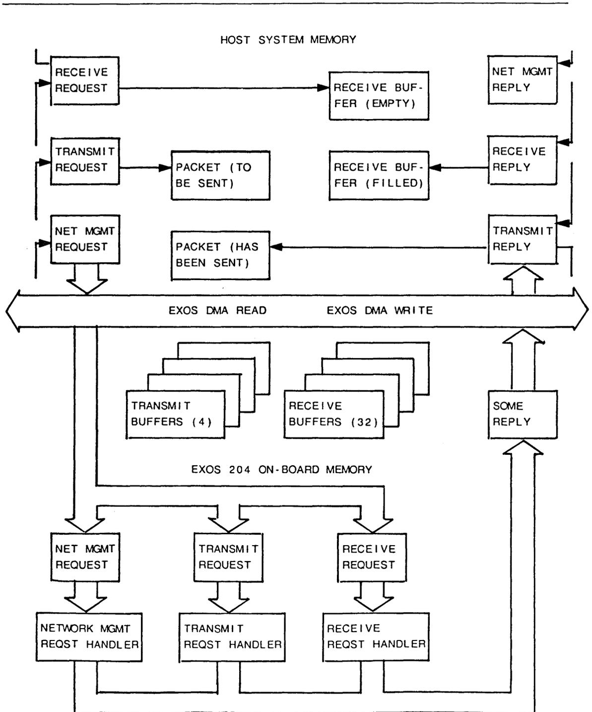
Figure 5-2: Link Level Controller Mode Request Processing Scheme
