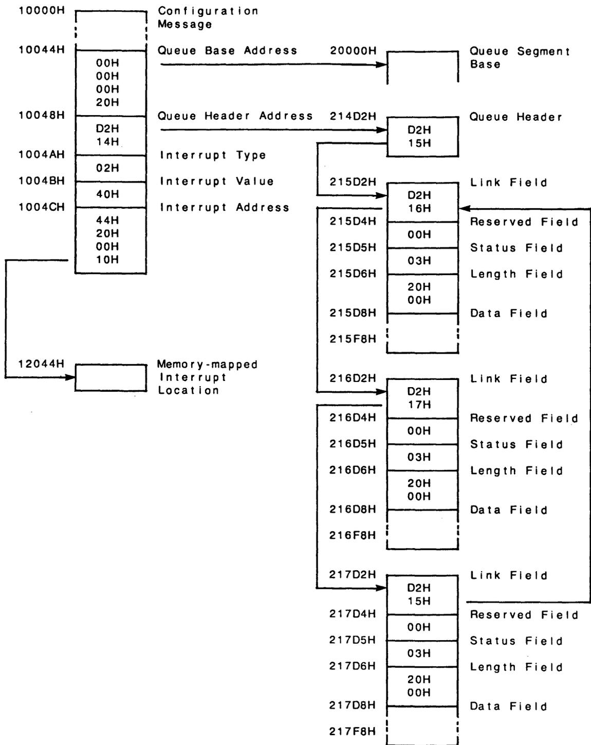
Figure 4-7: Example EXOS-to-Host Message Queue, at Initialization
