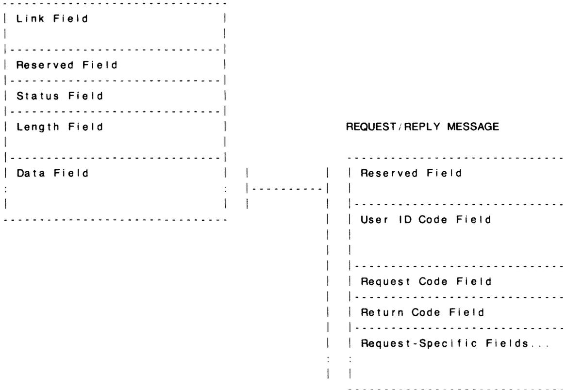
**Figure 5-1: Encapsulation of Request/Reply Message in Message Buffer**
