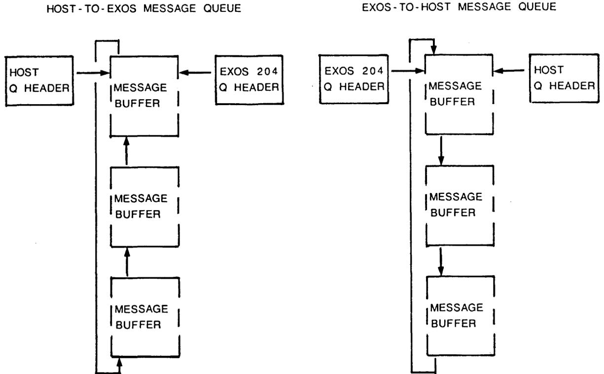
Figure 4-6: Message Queue Data Structures at Initialization Time
