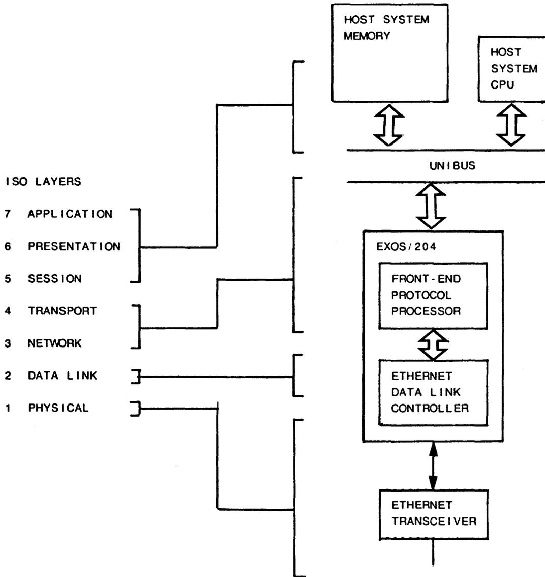
Figure 1-1: An EXOS 204 Front-End Processor Mode Implementation
