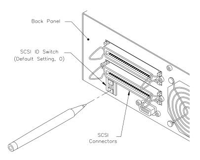
Figure 3-7 SCSI ID switch for the Mini Tabletop CTS
