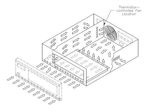
Figure 3-5 Air flow through the Mini Tabletop CTS
