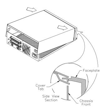
**2.** Rotate the top cover down and engage the flanges on the interior sides of the cover with the side panels of the Mini Tabletop CTS as shown. You may need to apply minimal pressure on the sides.
