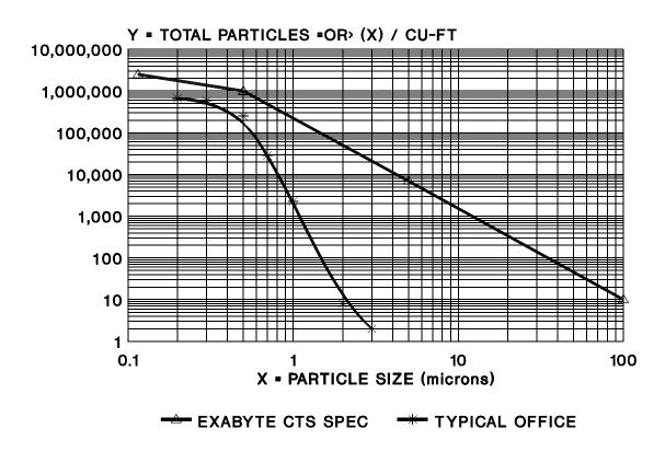
Figure 3-6 Particulate contamination specification vs. typical office
