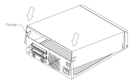
**3.** Using a #1 Phillips screwdriver, replace the screw on the back panel.
