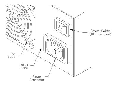
Figure 3-3 Power switch in the off position
