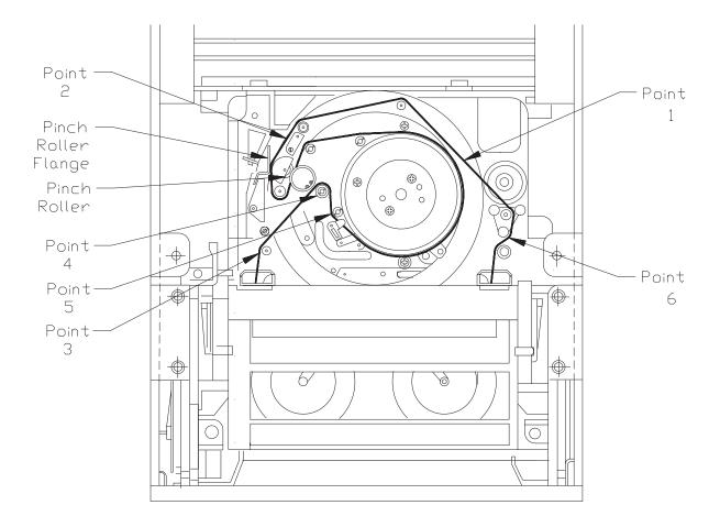
Figure 16-3 EXB-8500 with Tape Loaded (Tape Guide and Erase Head Bracket Removed)
