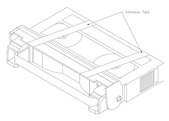
Figure 16-1 Taping Open the Data Cartridge Door
