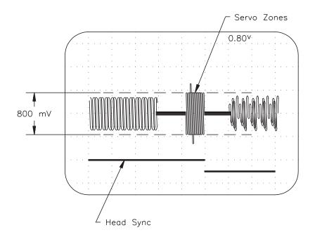
Figure 18-5 Oscilloscope Reading for EXB-8500 Format Servo Read Amplitude
