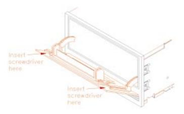
Figure 5-2 Separating the Door Parts (Front View of EXB-8500)
