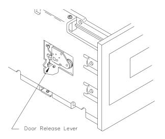
Figure 5-1 Location of Door Release Lever (Side View of EXB-8500)
