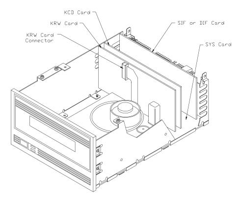
Figure 9-1 Edge Connector Mounted Cards
