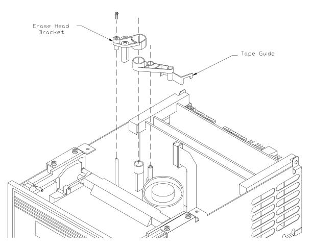
Figure 16-2 Location of Screw for Erase Head Bracket
