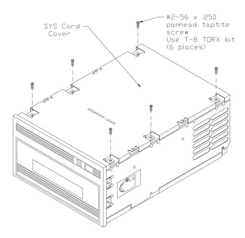
Figure 10-1 SYS Card Cover Screws (EXB-8500 Shown Upside Down)
