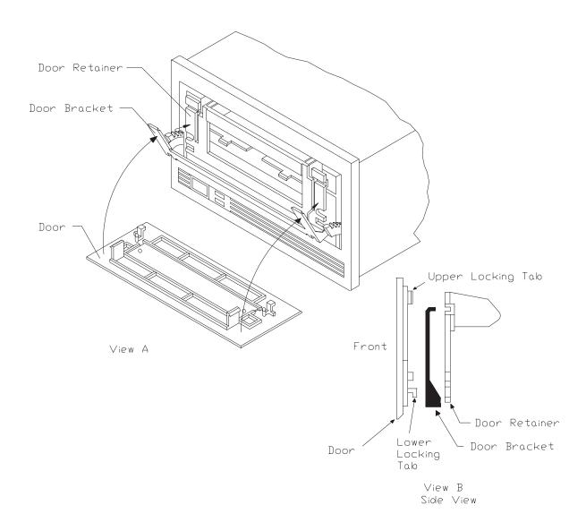
Figure 5-3 Position of Door, Door Retainer, and Door Bracket
