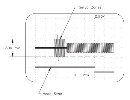
Figure 18-3 Oscilloscope Reading for EXB-8200 Format Servo Read Amplitude
