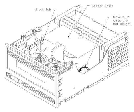
Figure 8-2 Correct Position of Deck Hanger's Copper Shield
