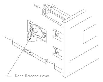
Figure 6-1 Location of Door Release Lever (Side View of EXB-8500)
