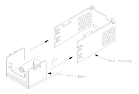
Figure 13-1 Removing the Main Housing
