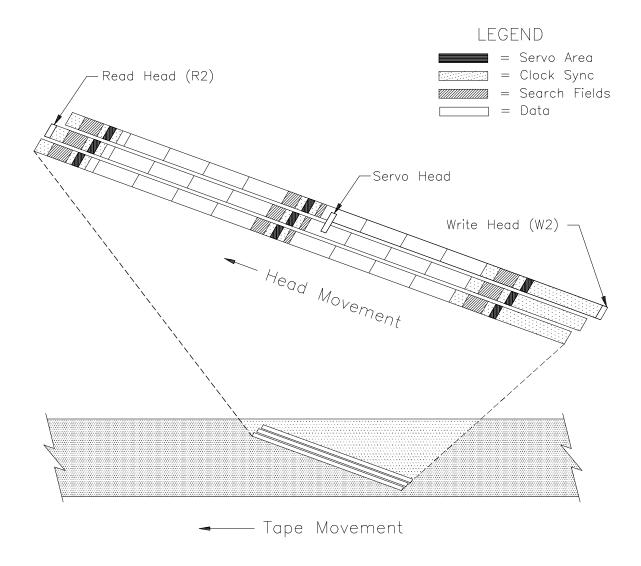
Figure 4-5 Position of the heads relative to the tracks (EXB-8200c format)
