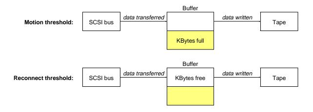
Figure 5-3 Motion and reconnect thresholds during a write operation
