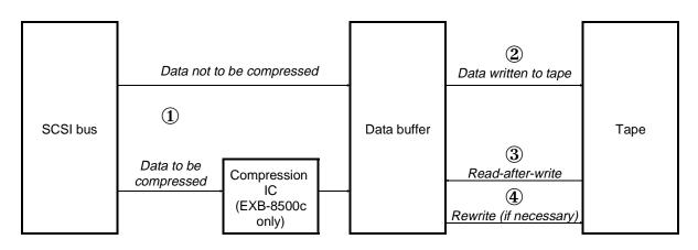
Figure 5-1 provides an overview of data flow during write operations.
