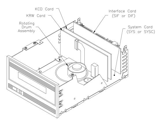
Figure 2-4 Internal components
