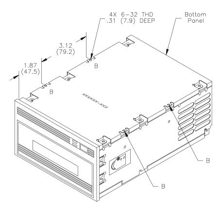
Figure 11-3 Mounting holes on the bottom
