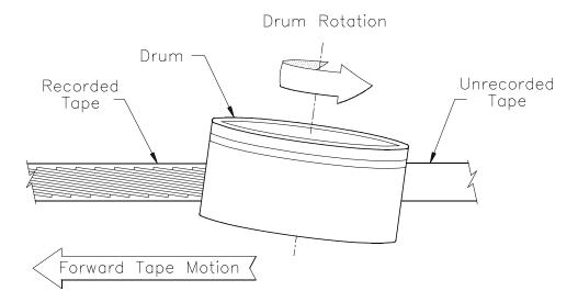
Figure 4-1 Helical scan recording
