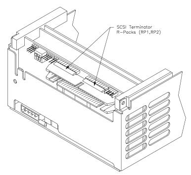
Figure 11-5 Resistor terminators on the single-ended EXB-8500 or EXB-8500c
