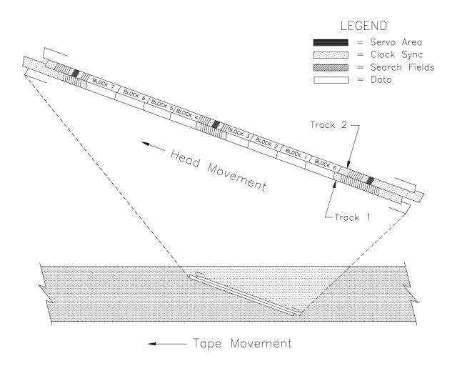
Figure 4-2 Physical track structure for EXB-8500/EXB-8500c format
