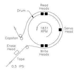
Figure 2-5 Write, read, and servo heads on the drum
