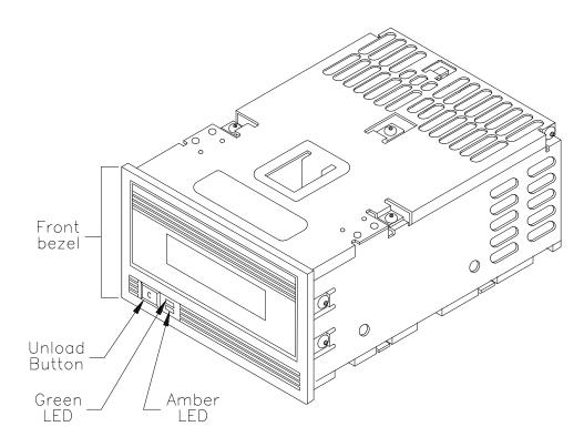
Figure 2-1 Front panel of the EXB-8500c
