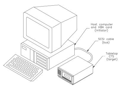
Figure 3-1 Physical connection in the SCSI environment (example)
