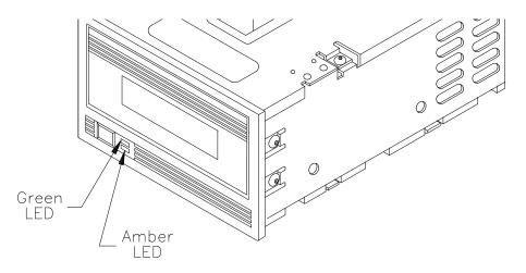
Figure 12-1 LEDs on the front of the EXB-8500
