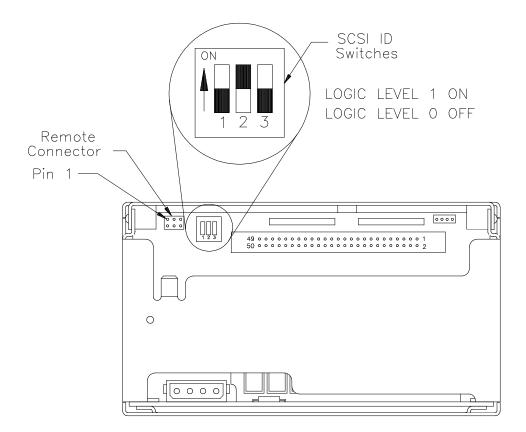
Figure 11-1 SCSI ID DIP switches and remote connector (single-ended configuration)
