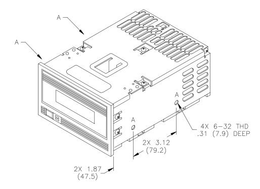
Figure 11-2 Mounting holes on the sides
