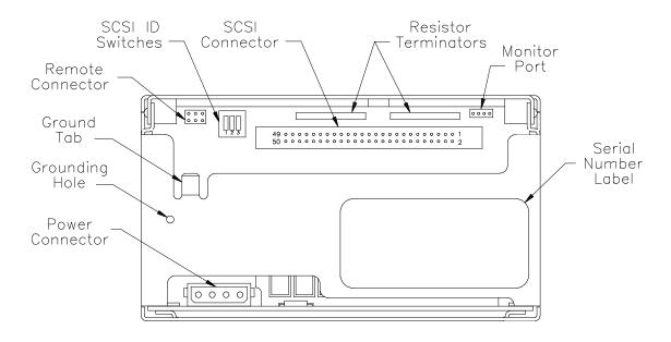
Figure 2-2 Back panel of the EXB-8500/EXB-8500c
