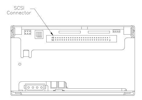
Figure 11-6 SCSI connector location
