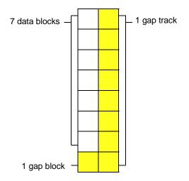
Figure 4-9 One gap block and one gap track in two physical tracks
