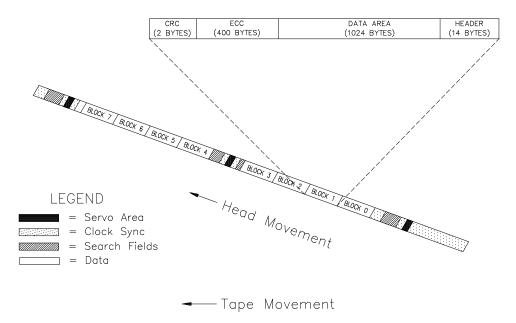
Figure 4-6 Physical block format (conceptual representation)
