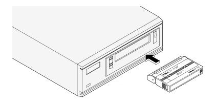
The tape drive loads the tape in approximately 20 seconds. When the middle LED is on, the tape drive is ready for read and write operations.
