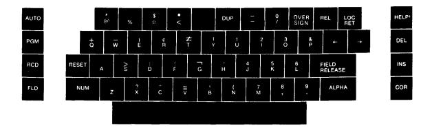
Figure 2-1 System 480 Keypunch Keyboard
