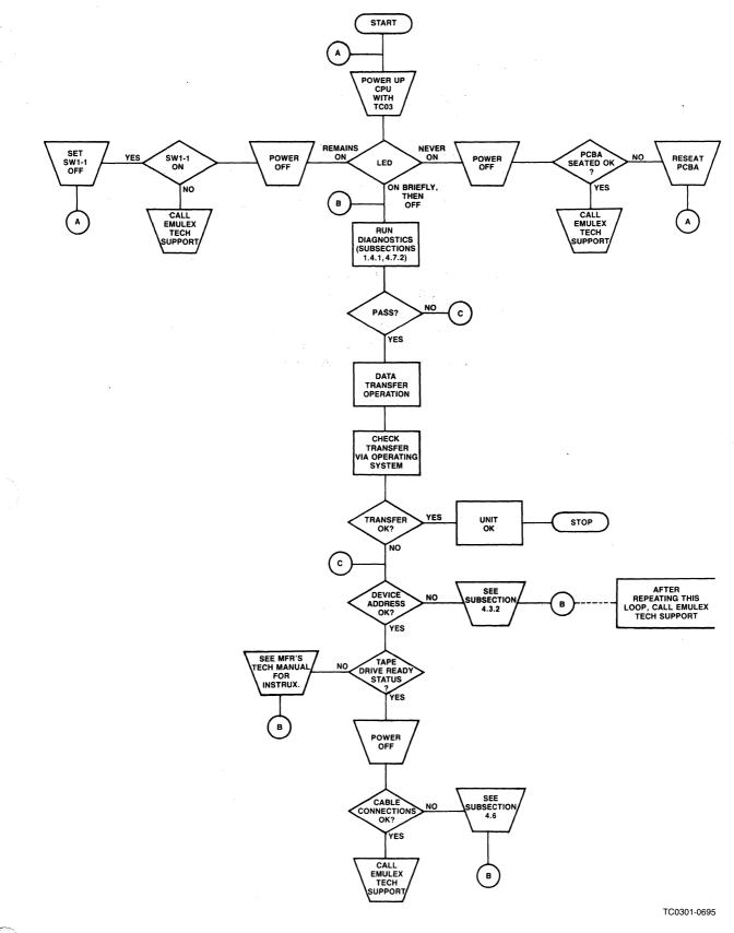
Figure 5-1. Fault Isolation Flowchart
