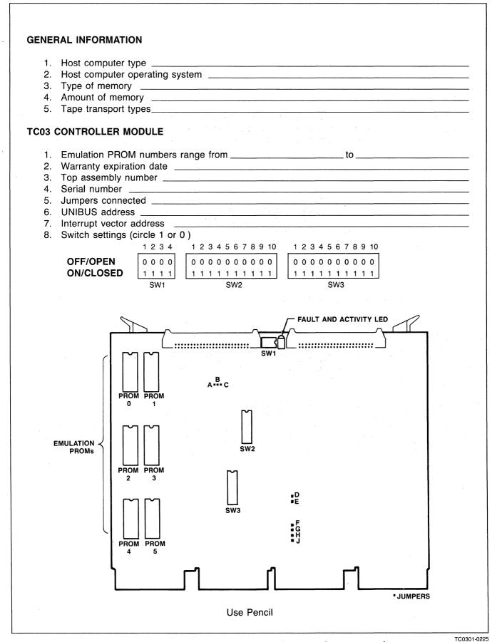
Figure 4-1. TC03 Configuration Reference Sheet
