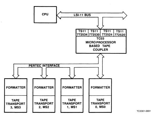
Figure 3-2. TCO3 Subsystem Logical and Physical Configuration
