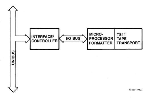
Figure 3-1. DEC TS11 Subsystem Logical and Physical Configuration
