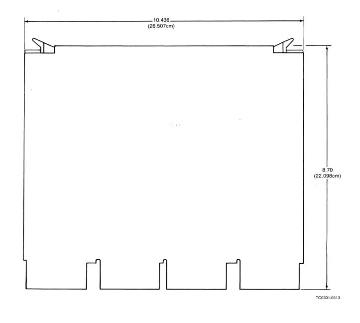
Figure 2-1. TC03 Tape Coupler Dimensions
