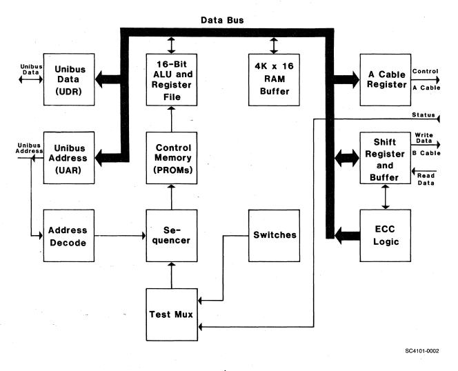
Figure 7-1. SC41/MS Block Diagram
