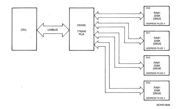
Figure 3-1. DEC MSCP Subsystem Logical and Physical Configuration
