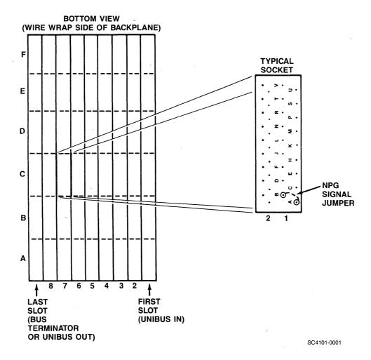
Figure 4-3. NPG Jumper Location
