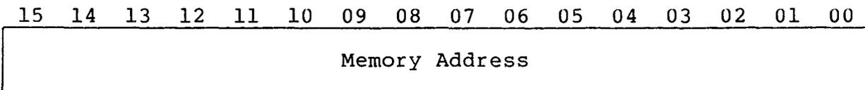
The RMBA register is initially loaded with the low-order 16 bits of the memory address for a data transfer. The low-order bit (00) is always forced to a zero. The RMBA register is incremented by two after transfer of a word to or from memory, unless the BAI bit is set.
