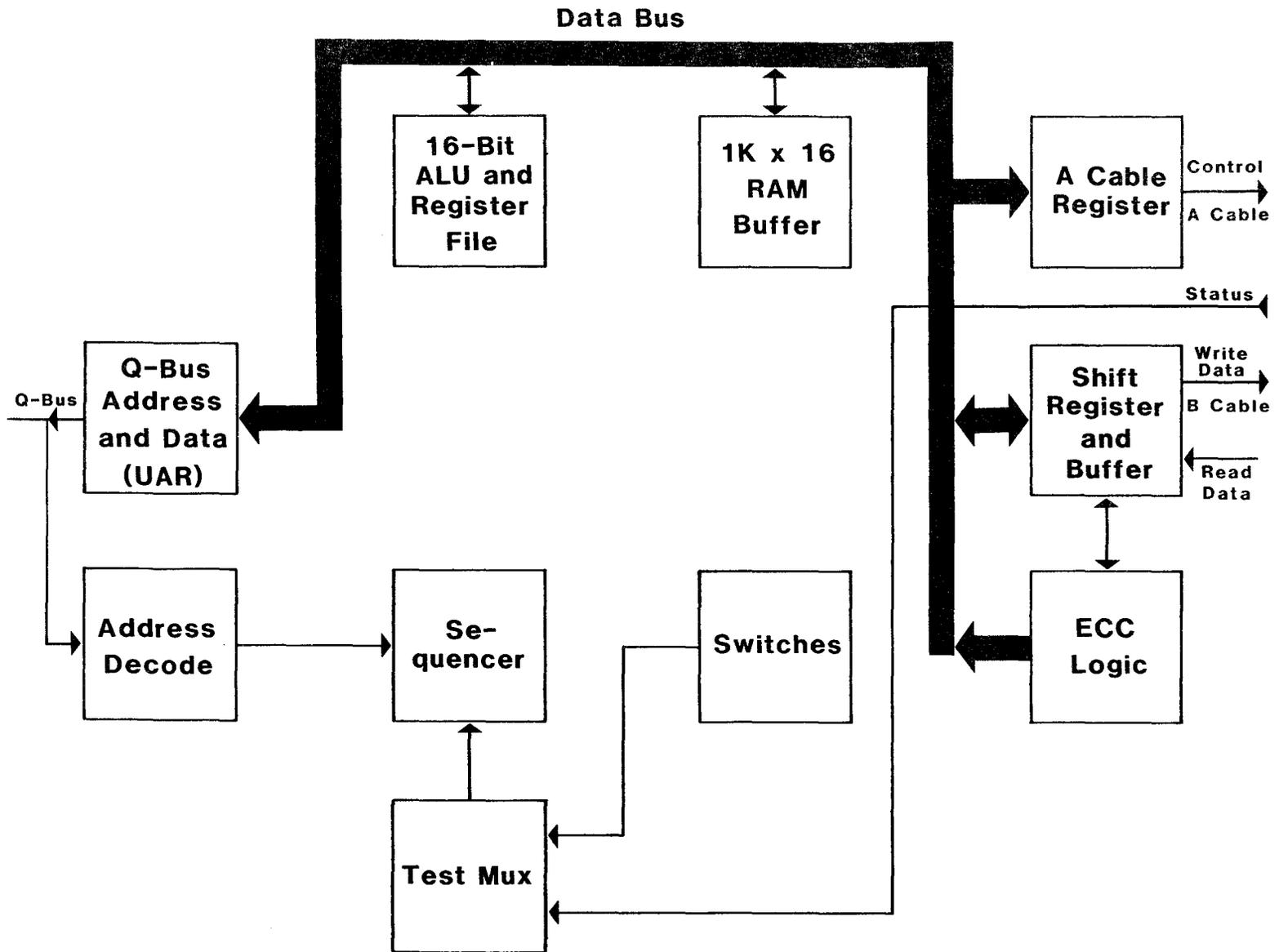
Figure 2-1 SC03 Block Diagram
