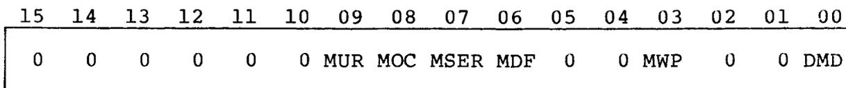
RMMR1 is a read/write register that allows a program to simulate various signals from the disk for diagnostic testing of the controller. The DMD bit must be set before any other bit has an effect on the controller. This register may be written into as a word or a byte. Writing to RMMR1 can occur at any time regardless of the status of the drive. A drive or controller clear resets this register except for bit 03, which is set.
