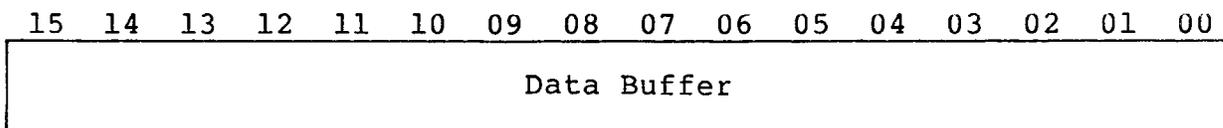
The RMDB register provides a maintenance tool to check the controller data paths. The IR (input ready) and OR (output ready) status indicators in RMCS2 registers are provided so that the programmer can determine when words can be read from or written into RMDB.
