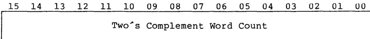
The RMWC register is loaded with the two's complement of the number of data words to be transferred to or from main memory. The register is incremented by one after each word transferred, and accommodates a maximum transfer of 65,536 words. The RMWC register is not cleared by INIT or controller clear.
