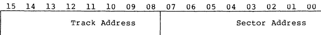
This register is used to address the sector and track on the disk to or from which a transfer is desired. It can only be loaded as a word. The RMDA is incremented each time a sector of data is transferred so that consecutive blocks are automatically addressed
