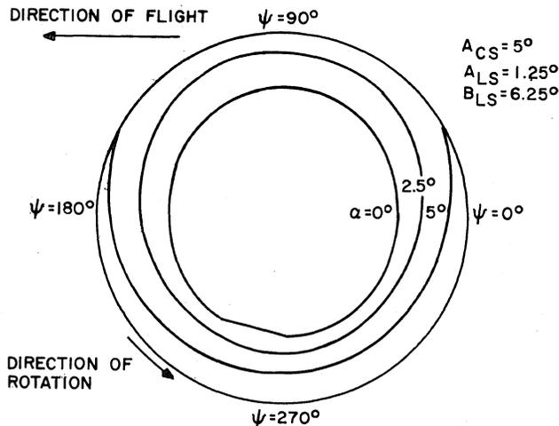
Figure 2: Non-Stall "Stick" Settings;  $A_{CS} = 5^\circ$ ,  $A_{LS} = 1.25^\circ$ ,  $B_{LS} = 6.25^\circ$
