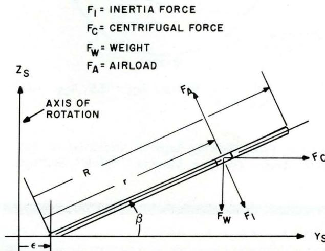
Figure 1: Side View Of Helicopter Rotor Blade
