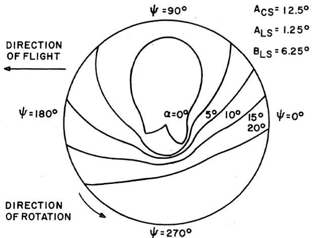
Figure 4: Stall "Stick" Settings;  $A_{CS} = 12.5^\circ$ ,  $A_{LS} = 1.25^\circ$ ,  $B_{LS} = 6.25^\circ$
