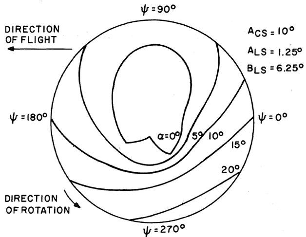
Figure 3: Stall "Stick" Settings;  $A_{CS} = 10^\circ$ ,  $A_{LS} = 1.25^\circ$ ,  $B_{LS} = 6.25^\circ$
