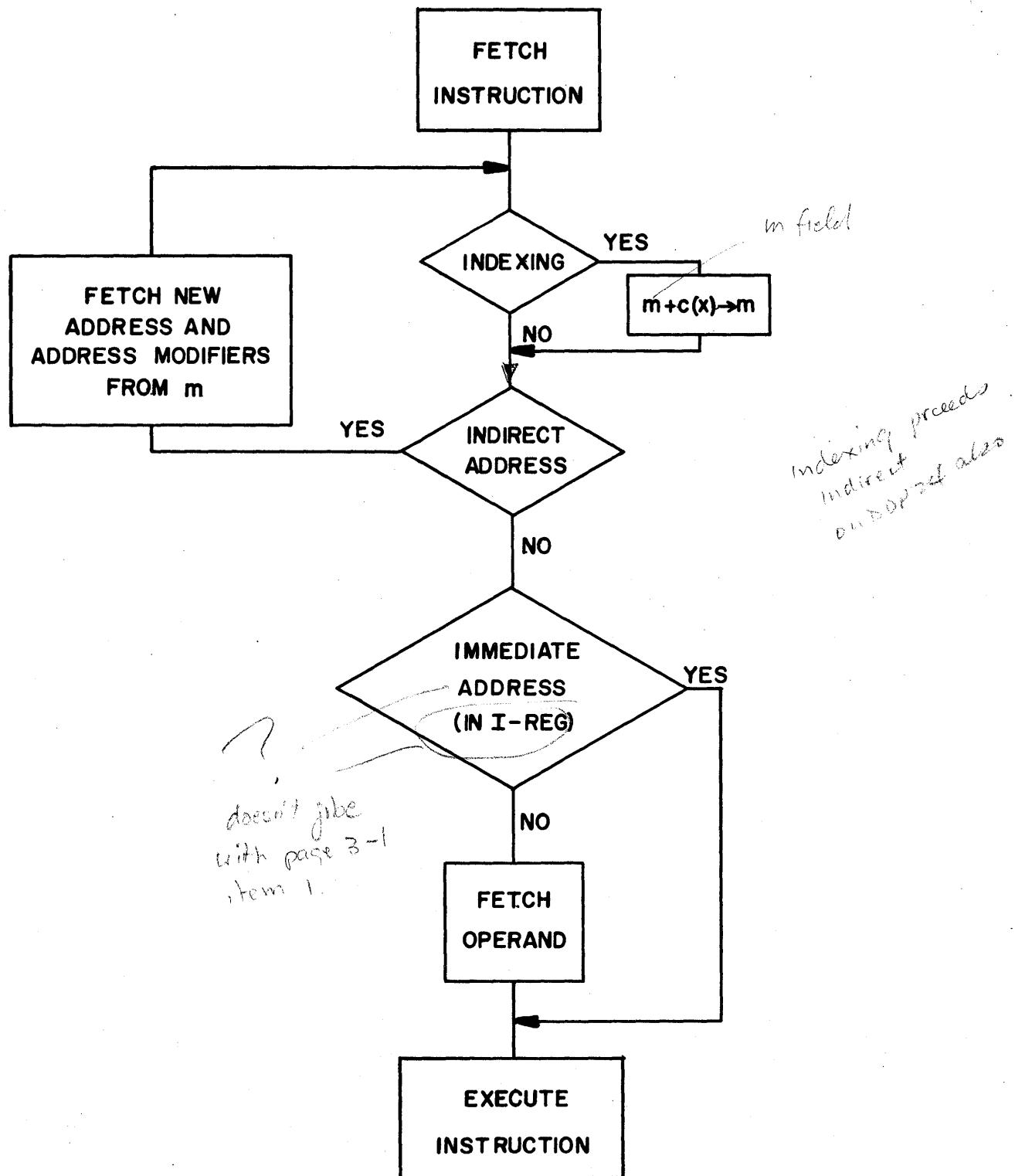
If both indirect addressing and address modification are specified, the modified effective address is used for indirect addressing at each level.
