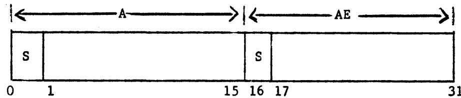
The AE Register is also used to hold 32 bit double length products and dividends of 16 bit Fixed-Point multiply/divide computation.
