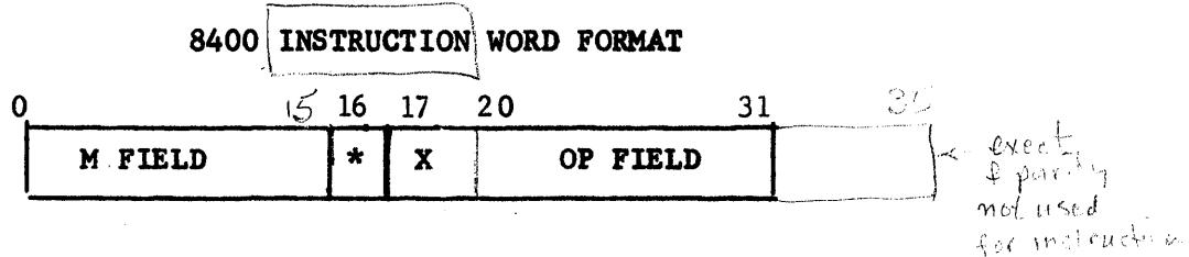
M is a 16-bit address field. \* is an indirect address bit.
