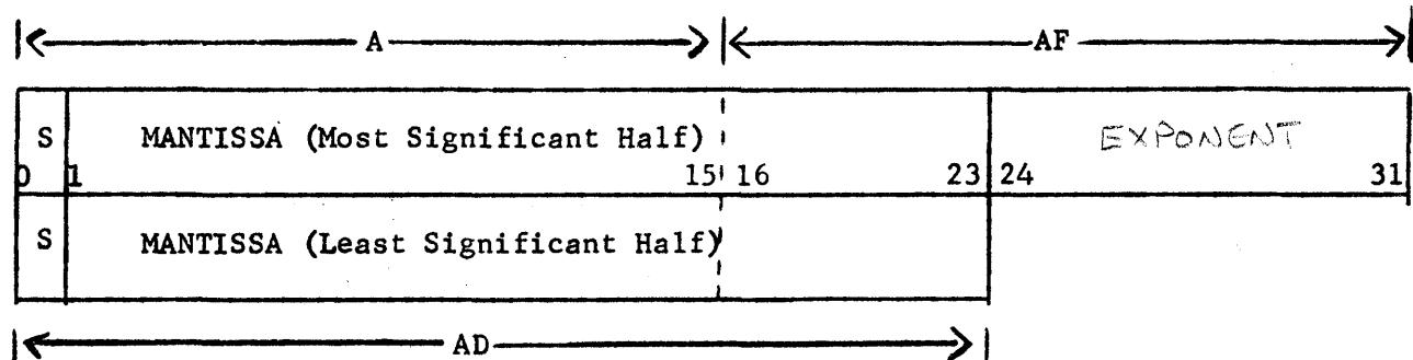
The AD Register is used to hold double precision products and dividends of single precision floating-point multiply/divide computations.
