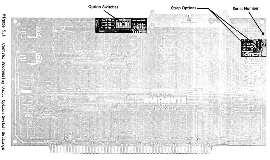
NOTE: The dots on the switches indicate the direction in which the switch should be set for correct operation.
