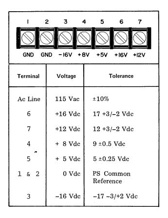
Figure 6.2 Power Supply Module Voltage Test Points, BS1
