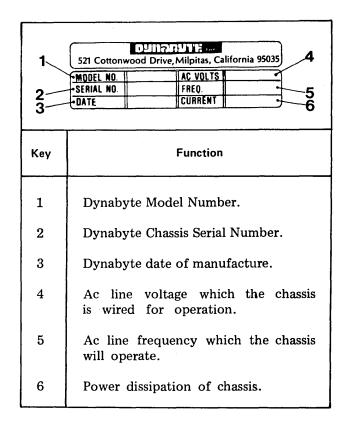
Figure 6.1 — Dynabyte Identification Plate
