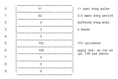
These parameters are correct for use with an ST506 drive.
