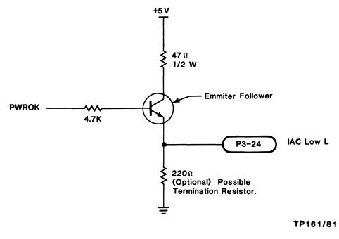
Figure 3-39. I-Bus Signal Line Driver Controller
