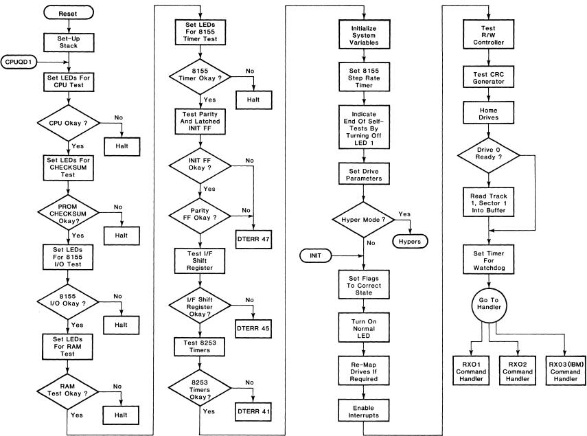
Figure 4-5. INIT Sequence in Microcode
