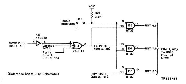
Figure 3-16. Interrupt Logic
