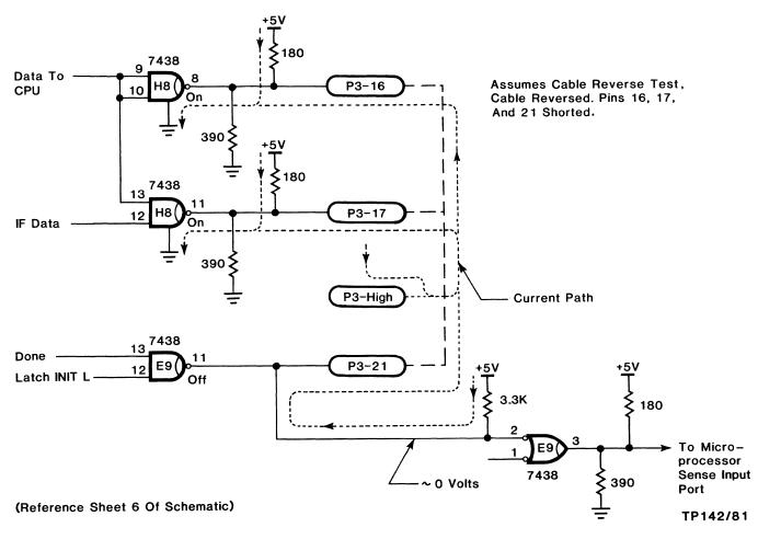
Figure 3-20. Cable Reversal Test Logic
