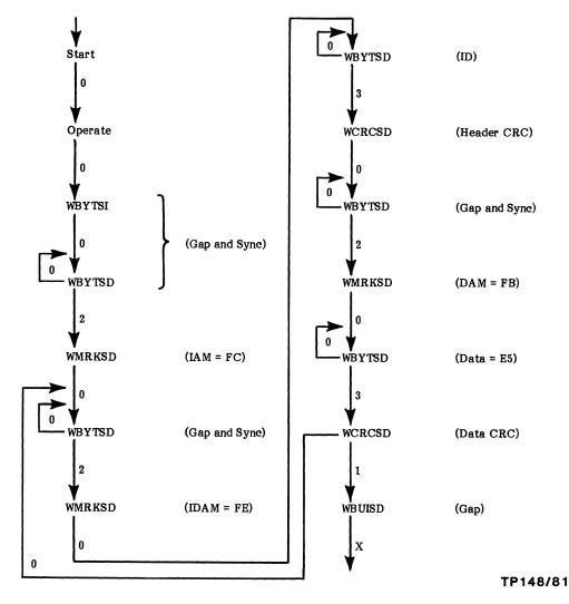
Figure 3-26. Functional Sequencing Example
