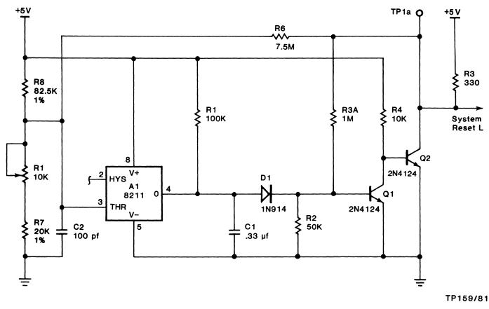
Figure 3-38. DC Power Up/Down Circuit
