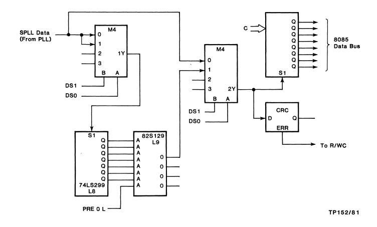
Figure 3-30. Read Serial Data Path
