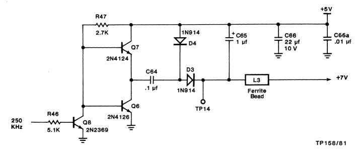
Figure 3-36. PLL Charge Pump Circuit
