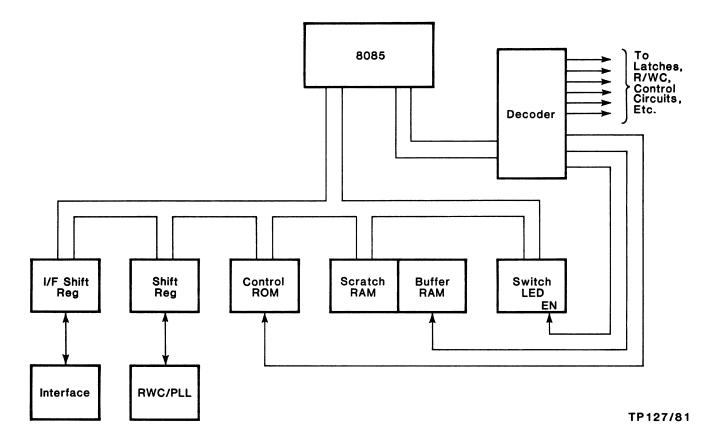
Figure 3-5. Master Controller Nucleus Block Diagram
