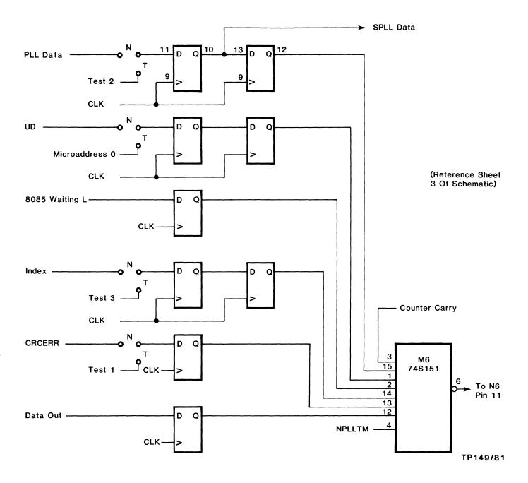
Figure 3-27. R/WC Branch Conditioning Circuitry
