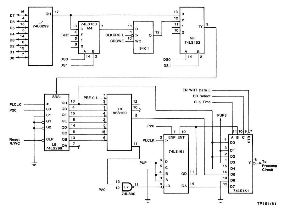
Figure 3-29. Write Serial Data Path
