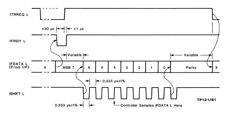
Figure 2-1. Timing, Interface to Controller
