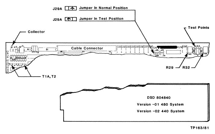
Figure 4-2. Controller Board Test Points and Jumpers
