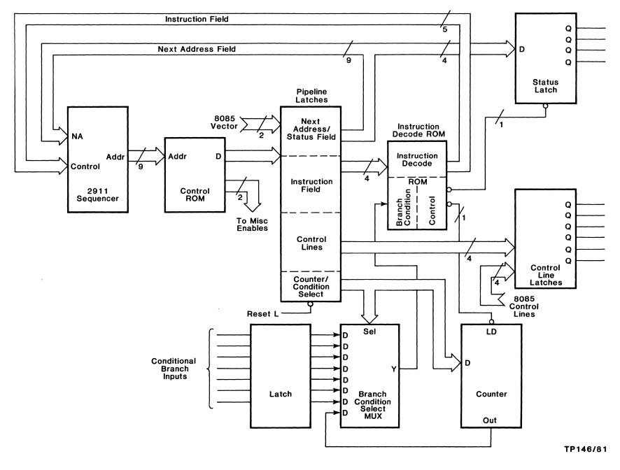
Figure 3-24. Read/Write Controller Block Diagram
