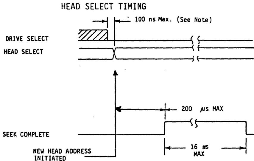
NOTE: If a head switch is not desired when drive is reselected, head select lines must be returned to the correct address no later than 100 n-sec after drive is reselected.
