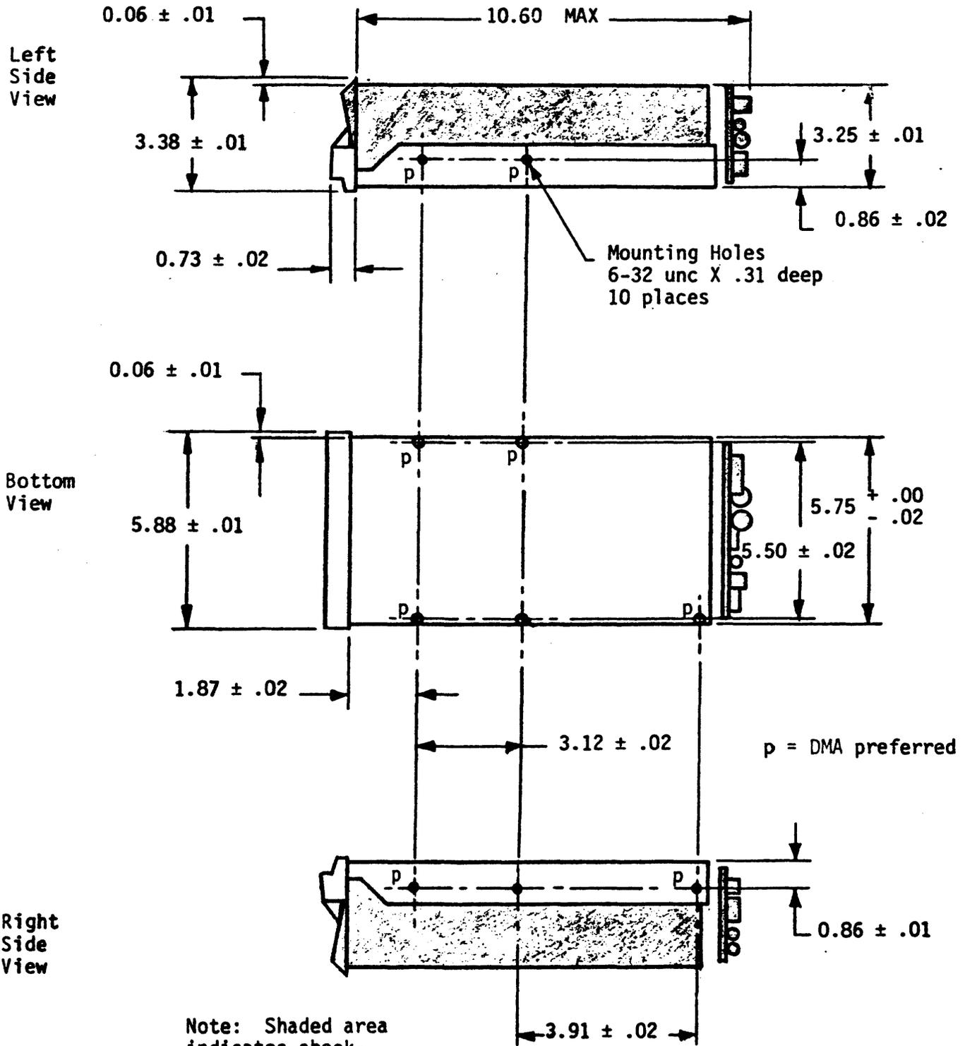
Note: Shaded area indicates shock-mounted portion of drive.
