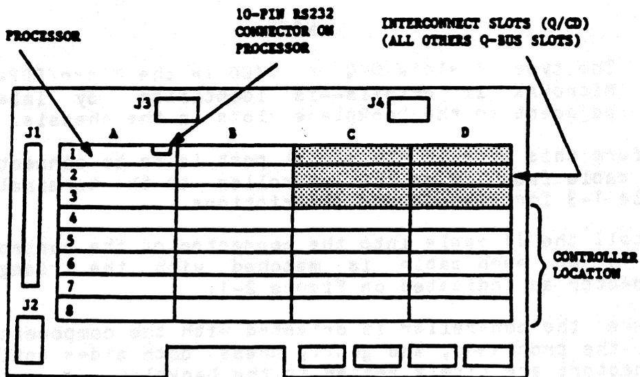
NOTE: Components on the board must be facing towards the Processor.
