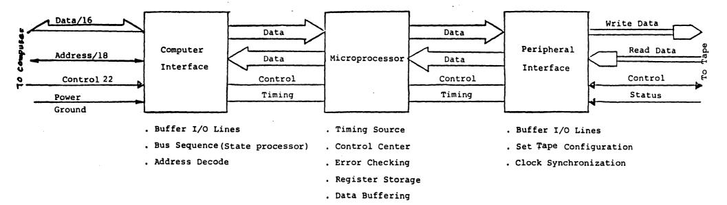
FIGURE 5-1: Simplified Block Diagram Peripheral Controller
