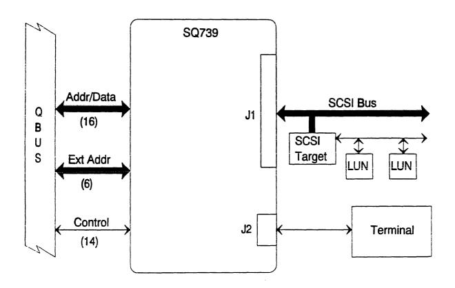
Figure 1 - SQ739 Simplified Diagram
