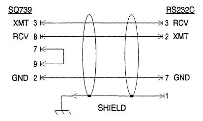
Figure 4 - Cable Pinout
