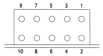
Figure 3 - Serial Port Connector
