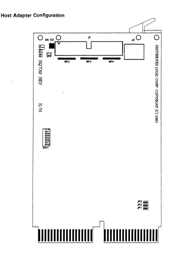
Figure 2 - SQ739 Host Adapter Configuration
