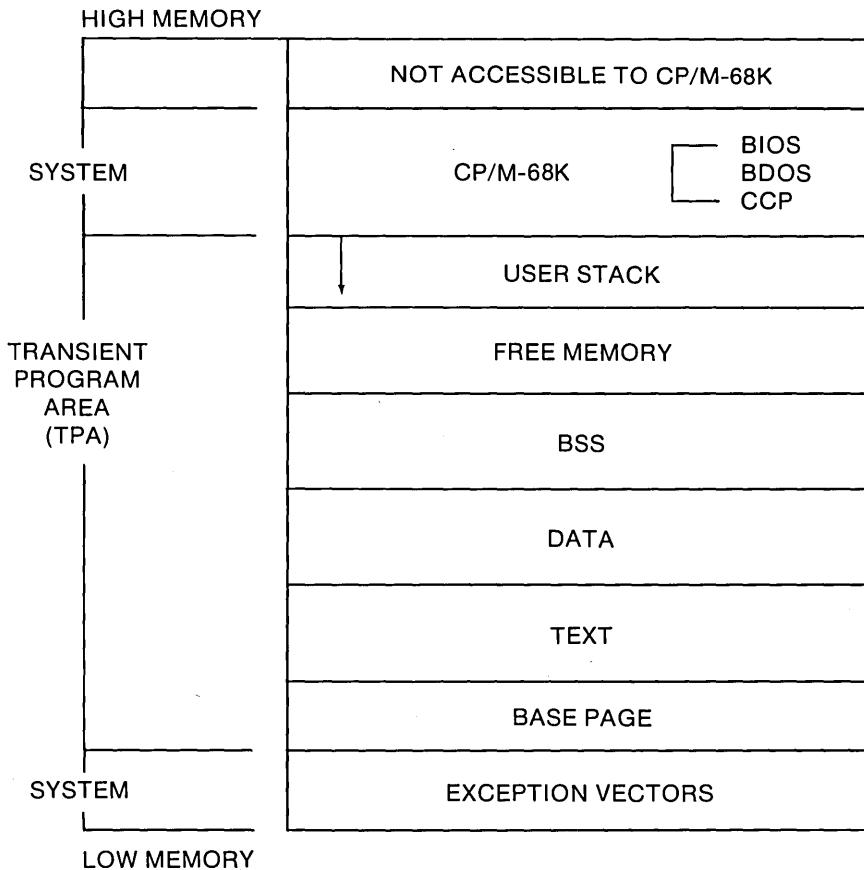
Figure 2-3. CP/M-68K Memory Model with Inaccessible Memory
