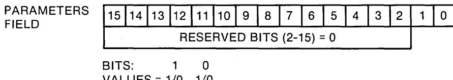
Figure 4-9. Parameters Field in TPAB
