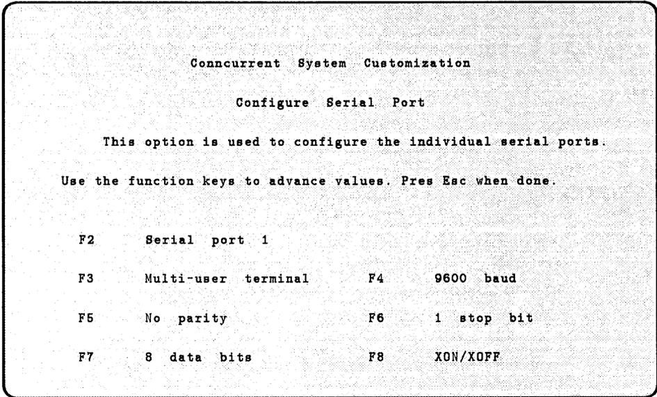
The above example reflects Port 1 set up as a Multi-user Terminal, at 9600 baud, No Parity, 1 stop bit, 8 data bits and software (XON/XOFF) handshaking.
