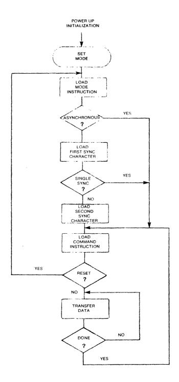
TYPICAL PROGRAMMING FLOWCHART AFTER POWER-UP RESET
