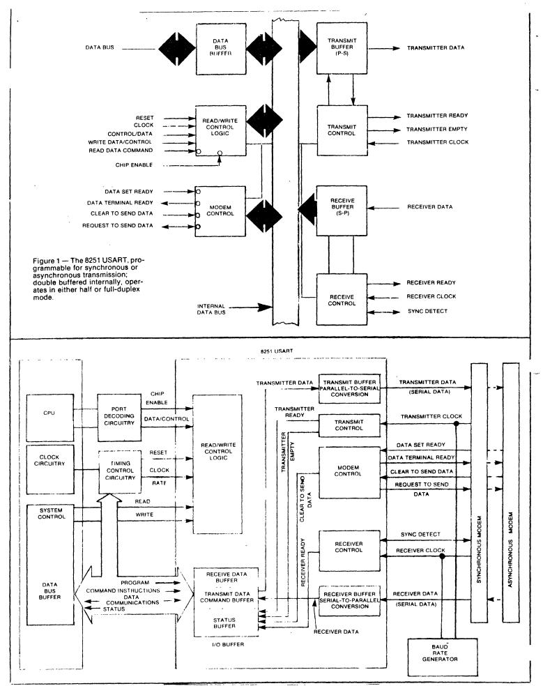
Figure 2 - 8251's implemented in a microcomputer system.
