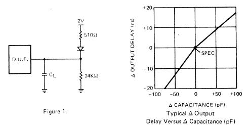
TEST LOAD CIRCUIT
