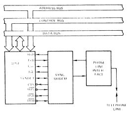
SYNCHRONOUS INTERFACE TO TELEPHONE LINES
