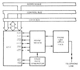
ASYNCHRONOUS INTERFACE TO TELEPHONE LINES
