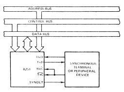
SYNCHRONOUS INTERFACE TO TERMINAL OR PERIPHERAL DEVICE
