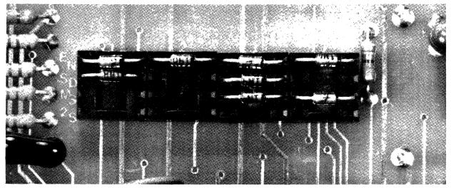
The following table shows which diodes are to installed for each be particular attribute. Diodes should be bent on .3" centers and then installed with the band to the right. (As viewed from the component side.)
