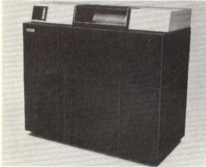
terchangeable print bands using a Universal Character Set Buffer, forms spacing through a forms control buffer, vertical line spacing at 6 or 8 lines per inch and a slew rate of up to 75 ips.
