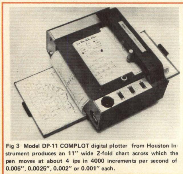
Fig 3 Model DP-11 COMPLIT digital plotter from Houston Instrument produces an 11" wide Z-fold chart across which the pen moves at about 4 ips in 4000 increments per second of 0.005", 0.0025", 0.002" or 0.001" each.
