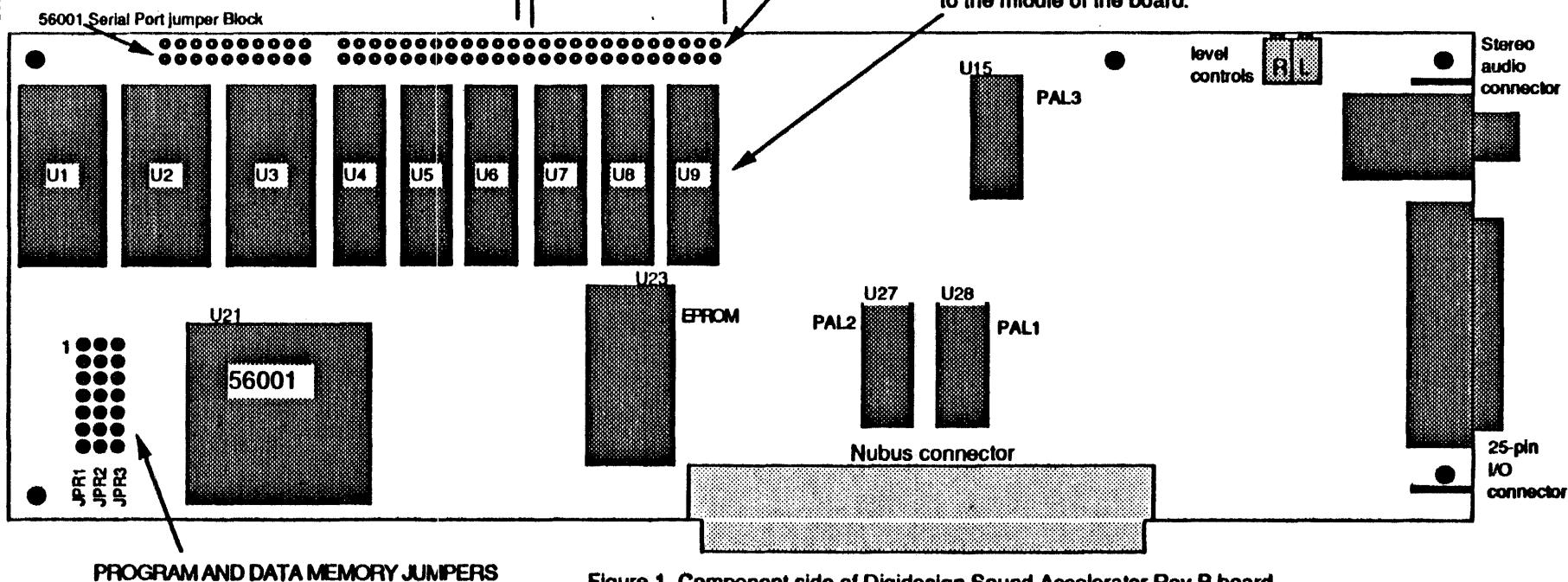
Figure 1. Component side of Digidesign Sound Accelerator Rev B board.
