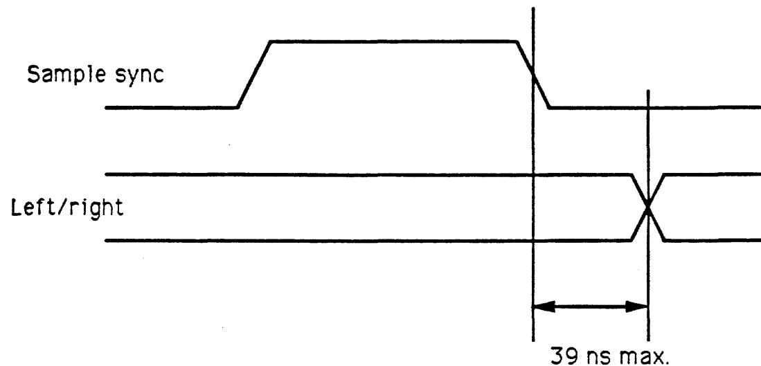
Figure ?. Timing for left/right signal.
