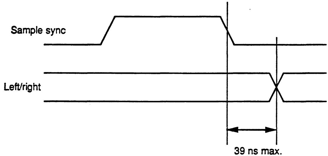
Figure 5. Timing for left/right signal.
