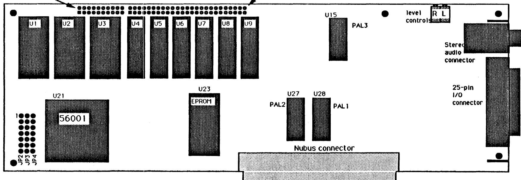
Figure 7. Component side of Digidesign Sound Accelerator board, Revision B.
