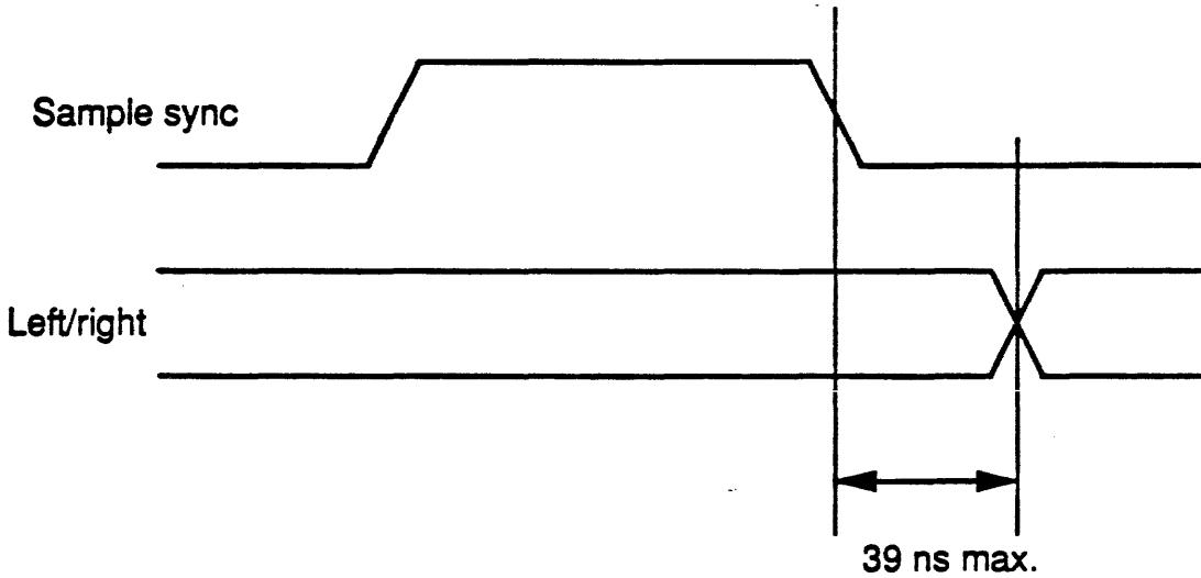
Figure 5. Timing for left/right signal.
