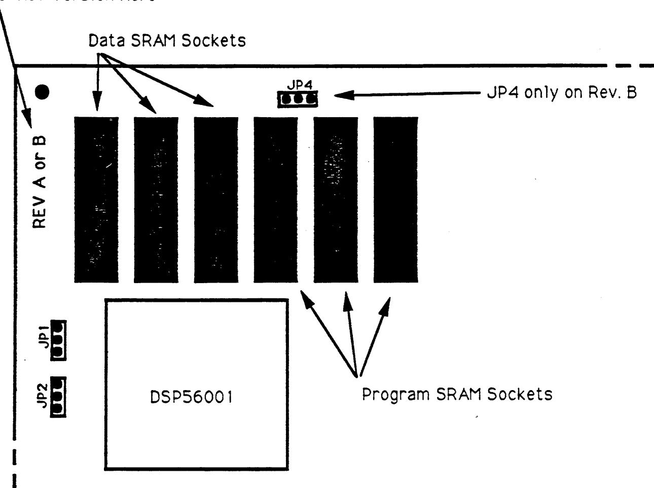
On Rev. A Audio Media boards both Data and Program SRAM may only be configured as either 8k X 24 or 32k X 24.
