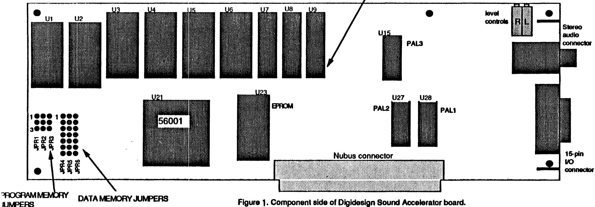
Figure 1. Component side of Digidesign Sound Accelerator board.
