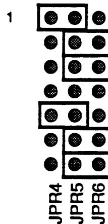
Figure 2. Data SRAM jumper settings
