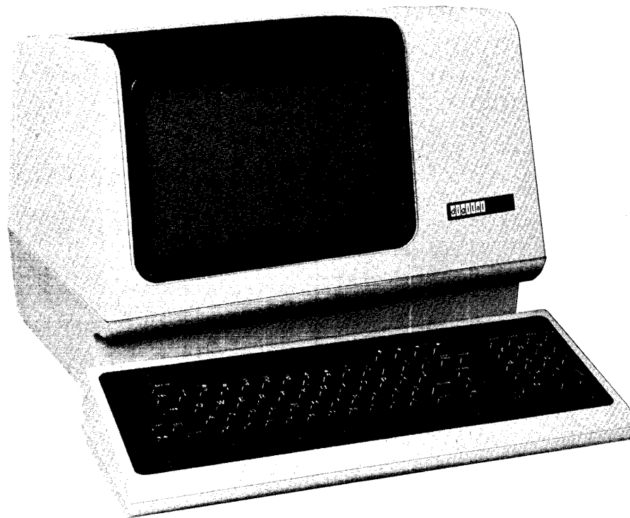
Figure 1-3 A VT100 Terminal
