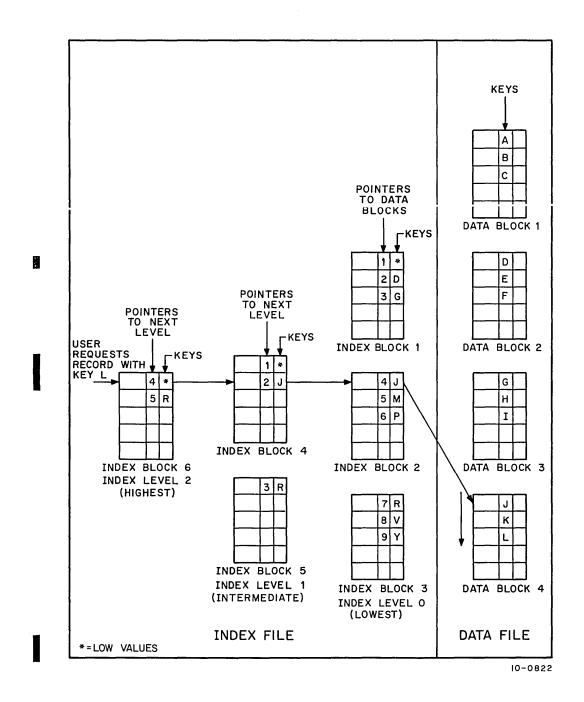
Figure H-1 Locating a Record in an Indexed Sequential File
