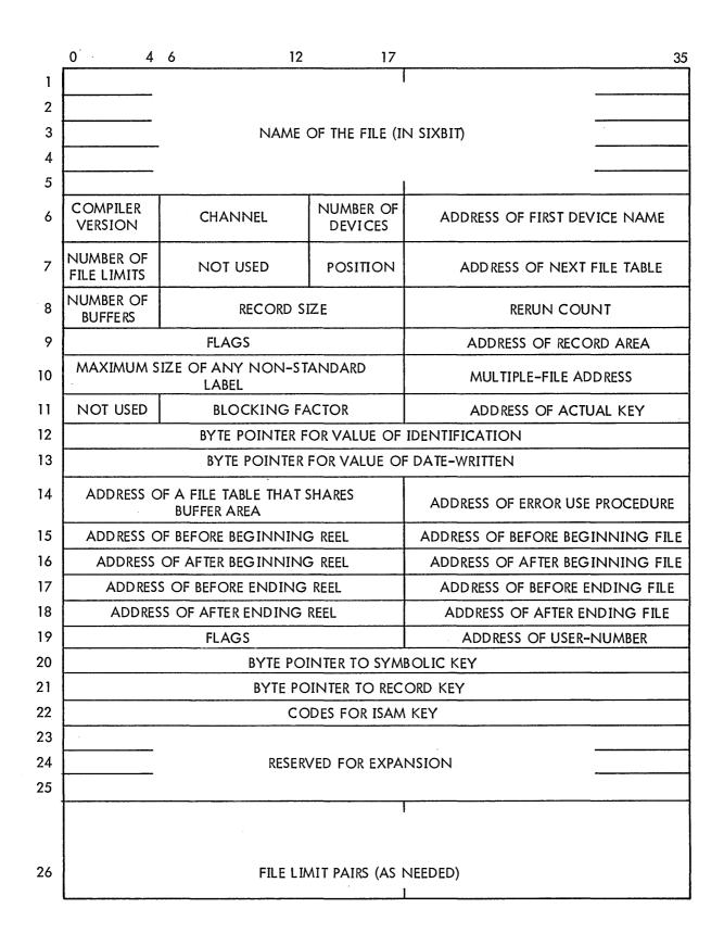
Figure 8-1 Structure of a File Table
