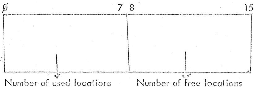
PUC: This routine will increment the PDL pointer, increment PDL counter left half, and decrement the PDL counters right half. It will actually make use of a subroutine PU to do this work, because all other PUSH-type instructions must do the same things to the pointer & counter.
