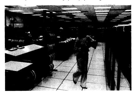
Here is an inside view of the University Computing Company's Dallas operations center. The photo shows multiple Univac 1108 computers which run UCC's EXEC/FASBAC and 1100/OS services. Other UCC services run with IBM and CDC systems.
