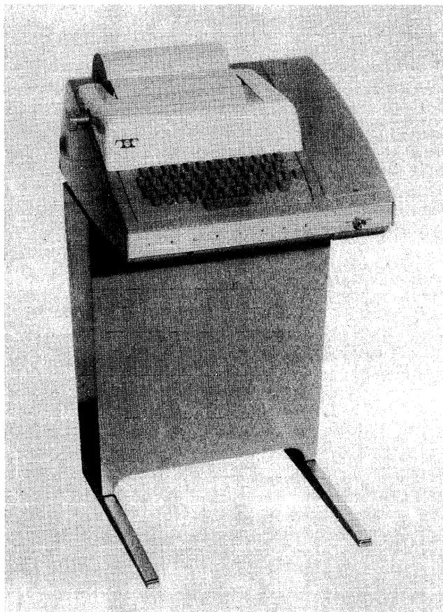
The Teletype Model 33 KSR (keyboard send/receive) terminal, because of its low cost and widespread software support, has long been the most popular choice among users of interactive time-sharing systems. It can be equipped with a paper tape reader and punch (which makes it an ASR unit) or a magnetic tape buffer. Alternatively, users can choose from a host of faster keyboard/printer terminals and CRT display units which are fully compatible with the Teletype terminals.
