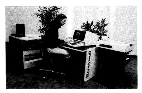
Honeywell's DPS 6 family of small computers includes the DPS 6/30, the 6/31, the 6/32 (pictured), the 6/34, and the 6/38 at the low end. Memory capacity for the systems ranges from 128K to 1024K bytes. Maximum disk storage capacity is from 10M to 1024M bytes. The systems accommodate a wide variety of printers ranging in speeds to 160 cps and 900 lpm. Purchase prices for the basic systems are \$19,500-\$30,000.
