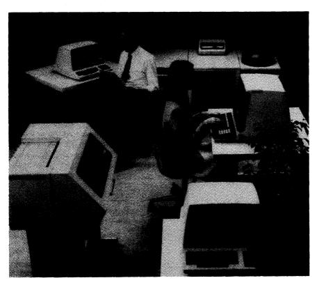
The MAI/Basic Four System 710 basic configuration consists of a central processor with 96KB of memory, one display terminal, two 35MB disk drives, and one 300 line-per-minute printer.
