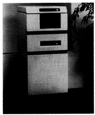
Features of the Plexus P/60 include multiprocessor architecture. During operation, the job processor performs data processing and operating functions while an intelligent mass storage processor handles disk and tape I/O, and intelligent communications processors handle terminal and printer I/O and data communications.
