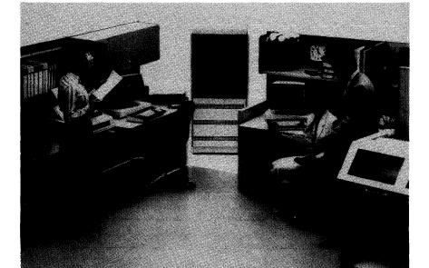
The Microdata Reality 4700 starts with a single base unit that can be configured by the user to meet a wide range of requirements. The base configuration includes 64KB of memory, 32MB of disk storage, and one single-density 1600 bpi streaming tape drive.
