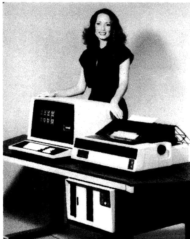
The MCM POWER is a multi-user system which supports up to 8 workstations. The system, which provides 64K bytes of main memory, also contains 256K bytes of virtual memory.
