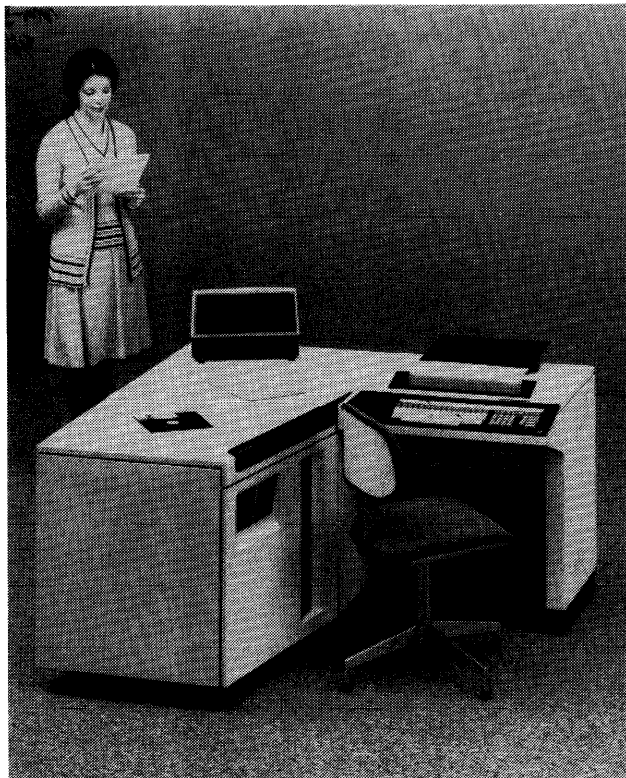
The Burroughs B 80, an impressive new small business computer, doesn't look like a typical minicomputer. Its processor is hidden inside the cabinetry and is part of a neatly packaged system. The entry-level configuration includes 32K bytes of MOS memory, a 60-cps printer and keyboard, two floppy disk drives (1 megabyte each), a magnetic tape cassette drive, and a 256-character visual display terminal. It can be purchased for $19,510.
