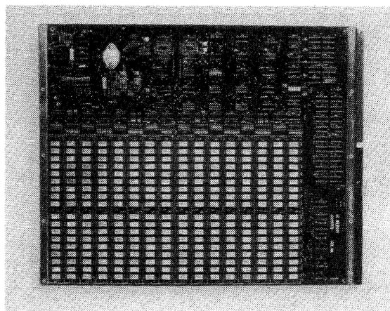
Here's Univac MCO's largest memory module: 65,536 16-bit words (1 megabit), with or without parity, on a single 15.6-by-15-inch board. Quoted at \$8,900 without parity and \$9,900 with parity, this dual-port NMOS memory has a cycle time of 660 nanoseconds and an access time of 560 nanoseconds.
