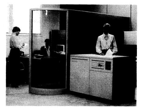
The 2200/201 is the entry-level model in Sperry's new 2200 Series of mid-range systems. The 2200/ 201 is equipped with 8 megabytes of main memory, expandable to 24 megabytes. Up to eight integrated disk drives can be added to the basic 2200/201 cabinet, which occupies only 10.5 square feet of floor space.
