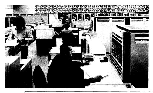
Two Model 45-III Processors are shown here, along with three card readers, six disc drives, and twelve magnetic tape units.
