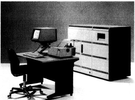
The 8890 system includes three IBM-compatible mainframes, each housed in a compact cabinet. In the front of the photo is one of Nixdorf's range of monochrome and color workstations for the 8890, plus a workstation printer.
