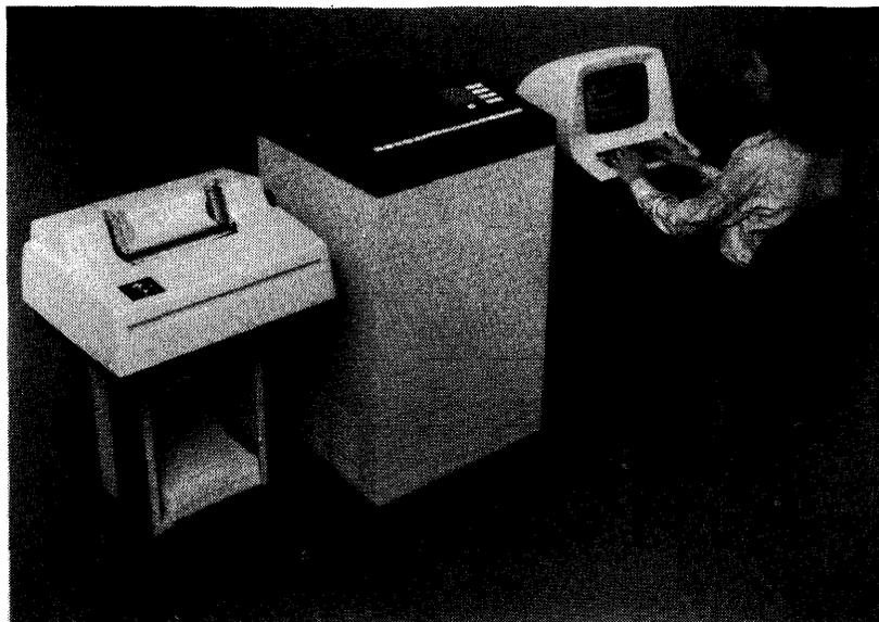
*The basic National CSS 3200 system includes the CPU, 256K bytes of error-correcting MOS memory, a byte multiplexer channel, and a CRT console terminal and console printer. The CPU also contains an air conditioning unit that permits the system to be used in a standard office environment.*
