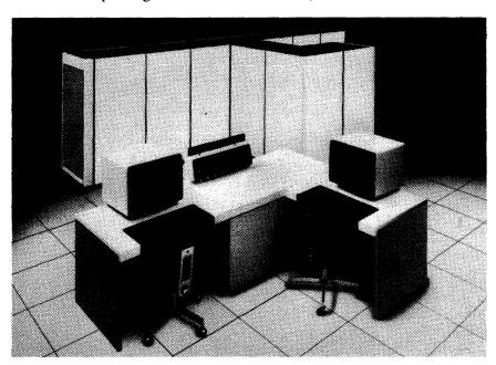
The large-scale AS/9000 Series is compatible with IBM's 3033 and 3081 systems. The basic AS/9000-2 system consists of a central processor with 12 megabytes of main memory, 64K bytes of buffer storage, 16 I/O channels, and a service processor console with 2 keyboard/display units and 2 floppy disk drives.
