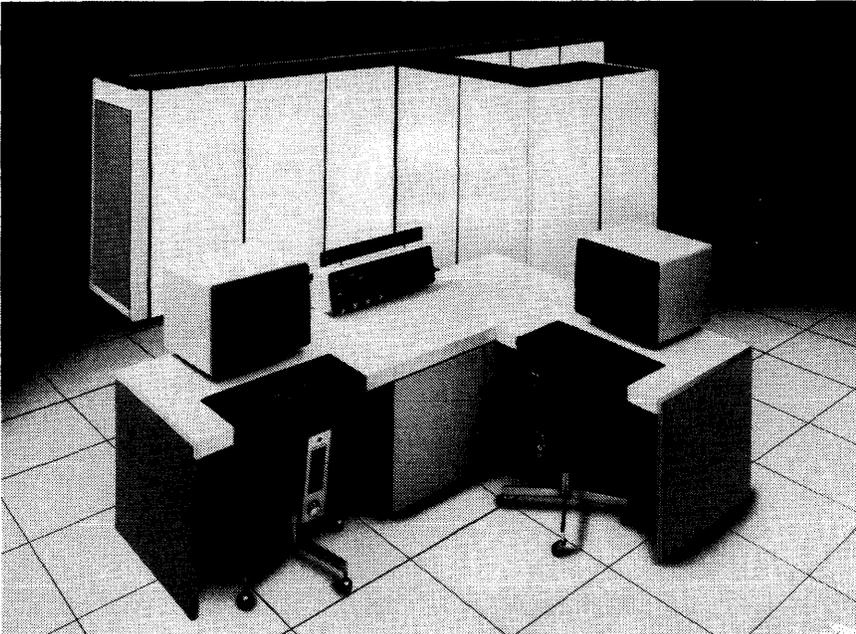
*The top-of-the-line AS/9000 Series is available in five processor models that are compatible with IBM's 3083, 3081, and 3084 systems. The AS/9000 Series processors have from 8 to 64 megabytes of main memory and from 6 to 32 I/O channels. The system console includes a service processor, two keyboard/display units, and two floppy disk drives.*
