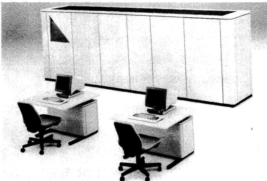
The recently announced top-of-the-line AS/XL Series is available in two processor models that are compatible with IBM's 3090 Series. The AS/XL Series processors have from 32 to 256 megabytes of main memory and from 16 to 64 I/O channels. The system features VLSI circuits throughout, and a one-megabyte dynamic working storage caching system between the main memory and the cache buffer.
