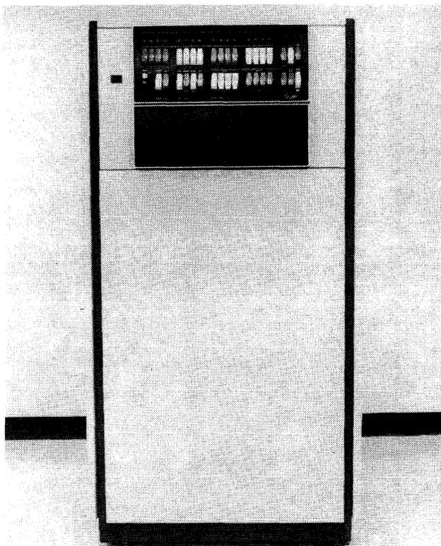
The Modcomp IV features a 32-bit-wide data path, memory addressing capacity of 1024K bytes, 2048 address mapping registers divided into 8 equal files of 256 each, and 32 direct memory processor channels. Double-density 600-nanosecond parity core memory modules are available.
